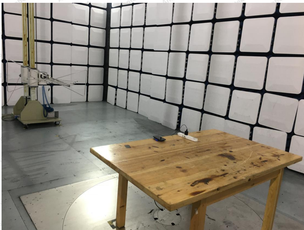
Photo of Radiation Emission Test
