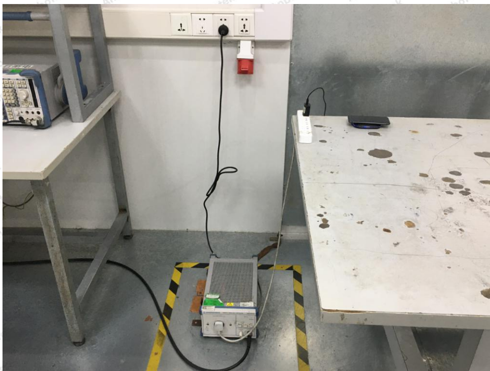
Photo of Conducted Emission Measurement
