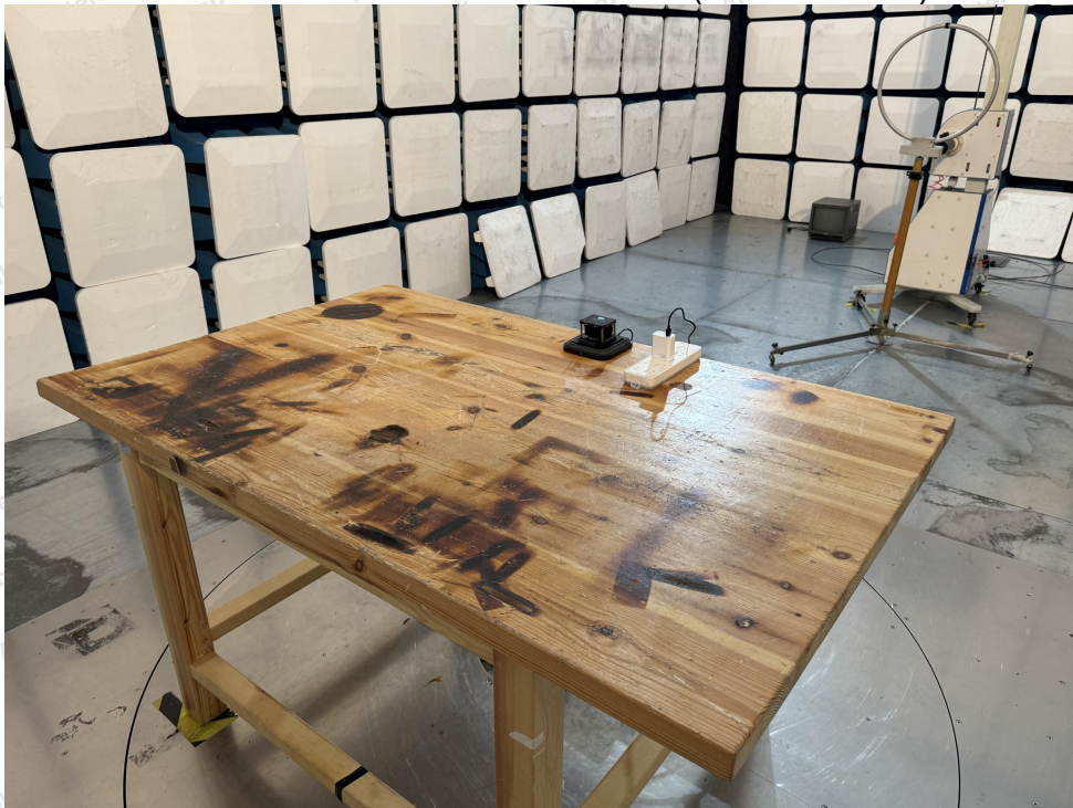
Photo of Radiation Emission Test (below 30MHz)
