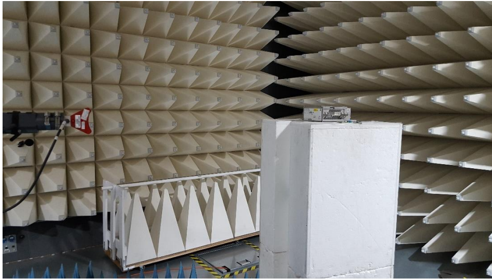
Figure C5. Radiated Emission High Range 18-40GHz test setup
