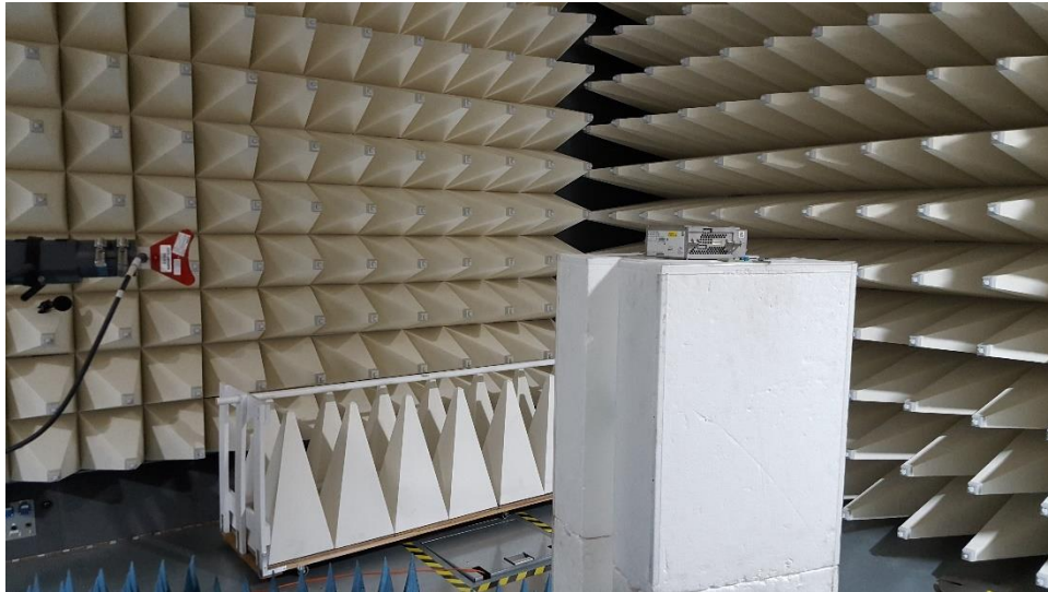
Figure C5. Radiated Emission High Range 18-40GHz test setup
