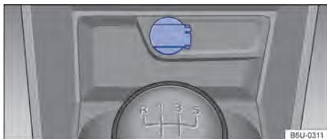
Fig. 103 In the front centre console: 12 V socket.
