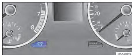
**Fig. 64** On the instrument cluster: headlight range control, instrument and switch lighting button.
