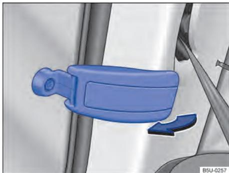
Fig. 53 Open the rear vent window.
