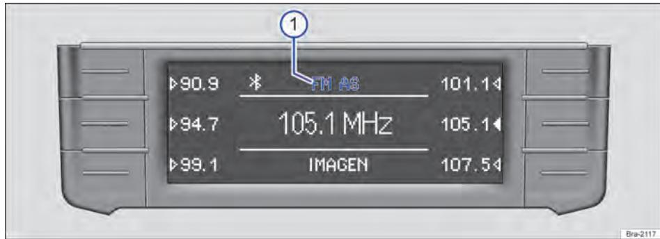
Fig. 137 RADIO main menu: displays frequency bands and memory levels.
