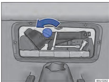
Fig. 163 Vehicle toolkit fastening handle.
