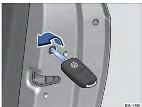
Fig. 45 Emergency vehicle locking with the vehicle key.
