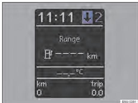
Fig. 79 On the instrument cluster: gearshift indicator (variable 2).
