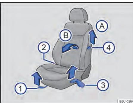
Fig. 57 On the front seat: controls.
