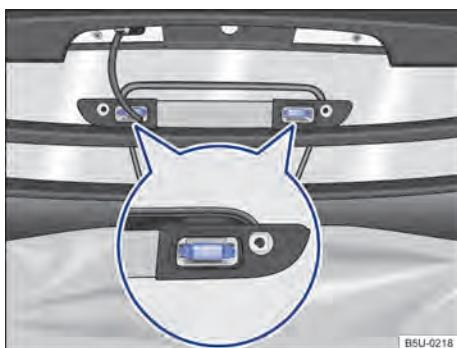
**Fig. 176** Elevated brake light: remove the bulb from the bed light.
