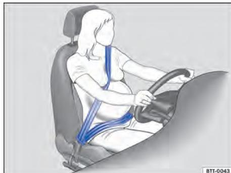
**Fig. 30** Correct seat belt routing during pregnancy.
