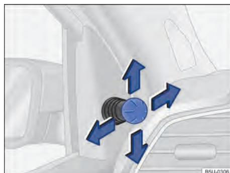
**Fig. 70** On the front doors: setting knob for the mechanical exterior mirrors.
