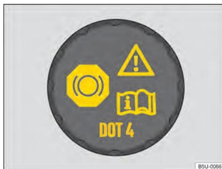
Fig. 192 On the engine compartment: brake fluid reservoir cap.
