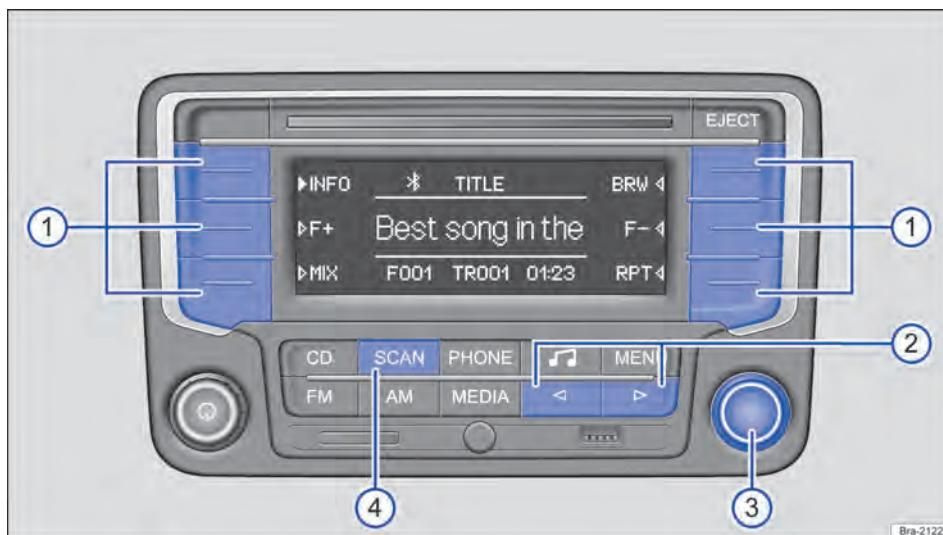
Fig. 147 Media playback display example: select playback modes.
