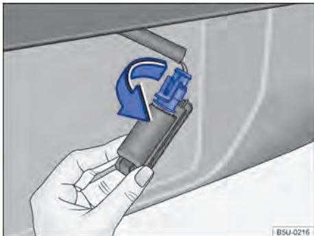
Fig. 174 Number plate light: remove the bulb socket.
