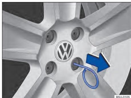
**Fig. 202** Removing the wheel bolt caps.
