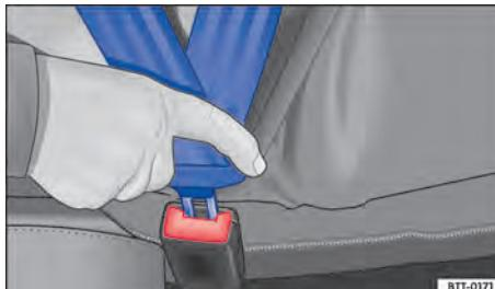
Fig. 27 Inserting the seat belt latch plate into the buckle.
