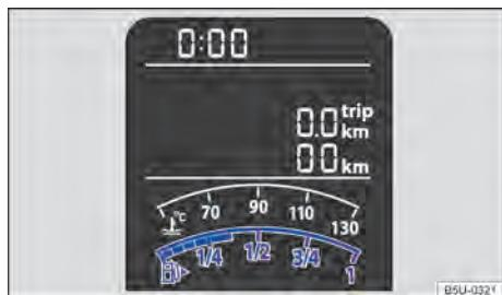
Fig. 12 On the instrument cluster display: fuel gauge (variable 1).
