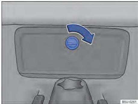
Fig. 162 On the rear seat floor: access to the vehicle toolkit housing.
