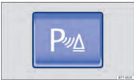
**Fig. 88** On the upper part of the centre console: parking distance control on/off button (Park Pilot).
