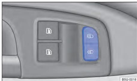
Fig. 42 On the driver door: central locking button.
