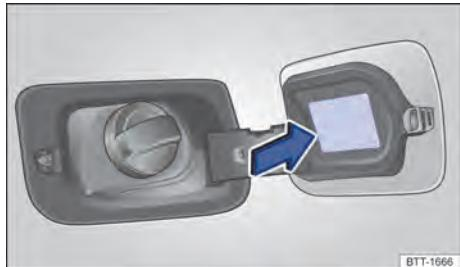
Fig. 197 On the inner side of the fuel tank flap: tyre pressure label.
