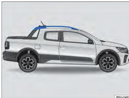
**Fig. 157** Roof rack longitudinal supports (both sides).
