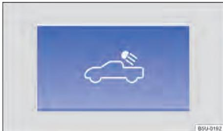
Fig. 65 On the centre console: bed lighting button.
