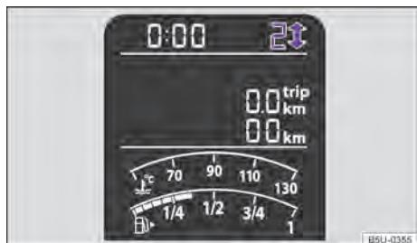
Fig. 78 On the instrument cluster: gearshift indicator (variable 1).
