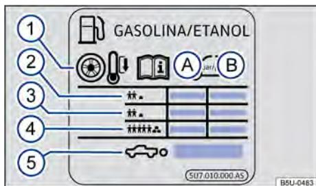
Fig. 196 Sticker with the tyre pressures.
