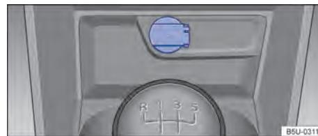
Fig. 105 In the front centre console: 12 V socket.
