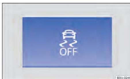
**Fig. 92** On the centre console: manual ASR on/off button.
