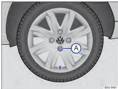
Fig. 203 Removing the wheel covers.
