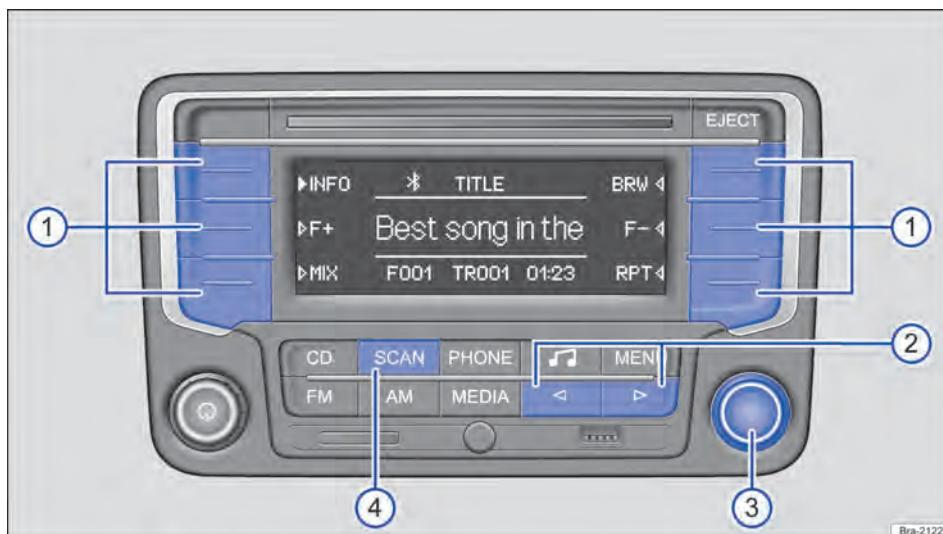
Fig. 145 Media playback display example: MP3 storage location displayed when changing tracks.
