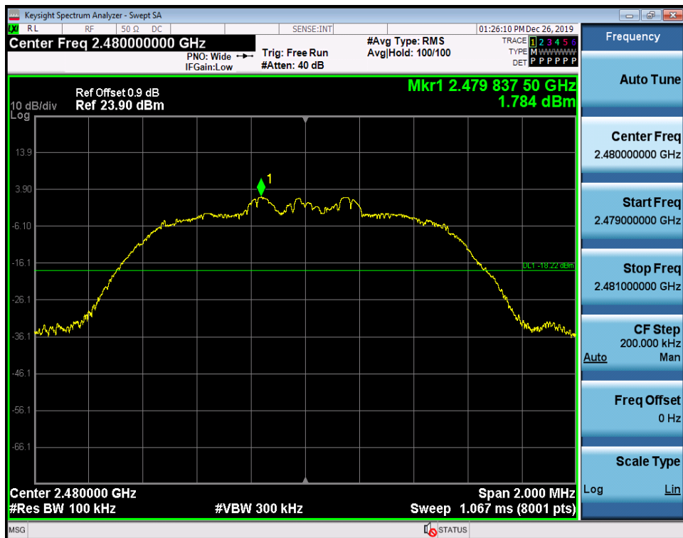
RF Conducted Spurious Emissions_2DH5_2480
