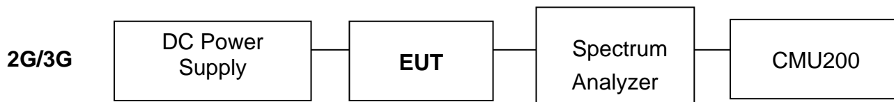
Fig. 2-1 Configuration of Tested System (Fixed Channel-Conducted)
