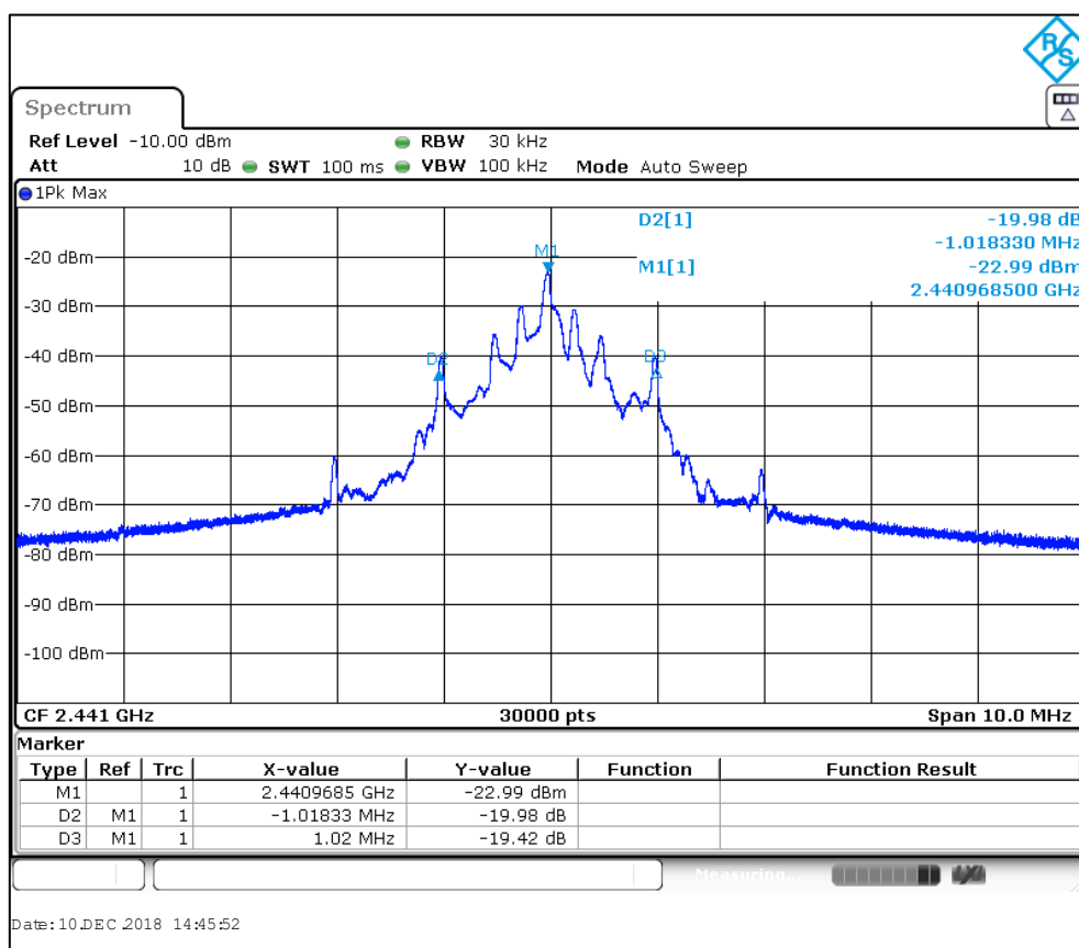
Figure 31. 20 dB bandwidth at 2441 MHz.
