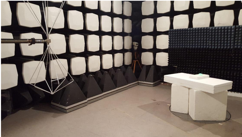
Photo 3 - Radiated emission test setup for 30 - 200 MHz.
