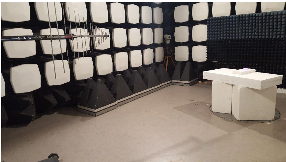
Photo 4 - Radiated emission test setup for 200 - 1000 MHz.
