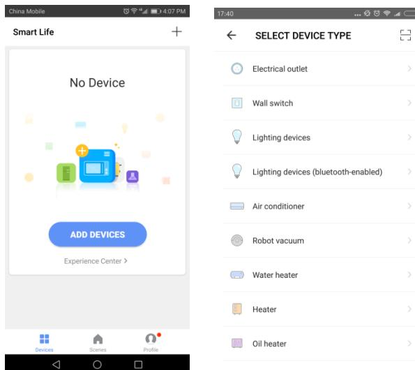
**Step 2:** Switch on power supply. The light will blink rapidly. If not, press the "reset" button on the wifi controller. Click "Confirm light rapidly blink" to continue.
