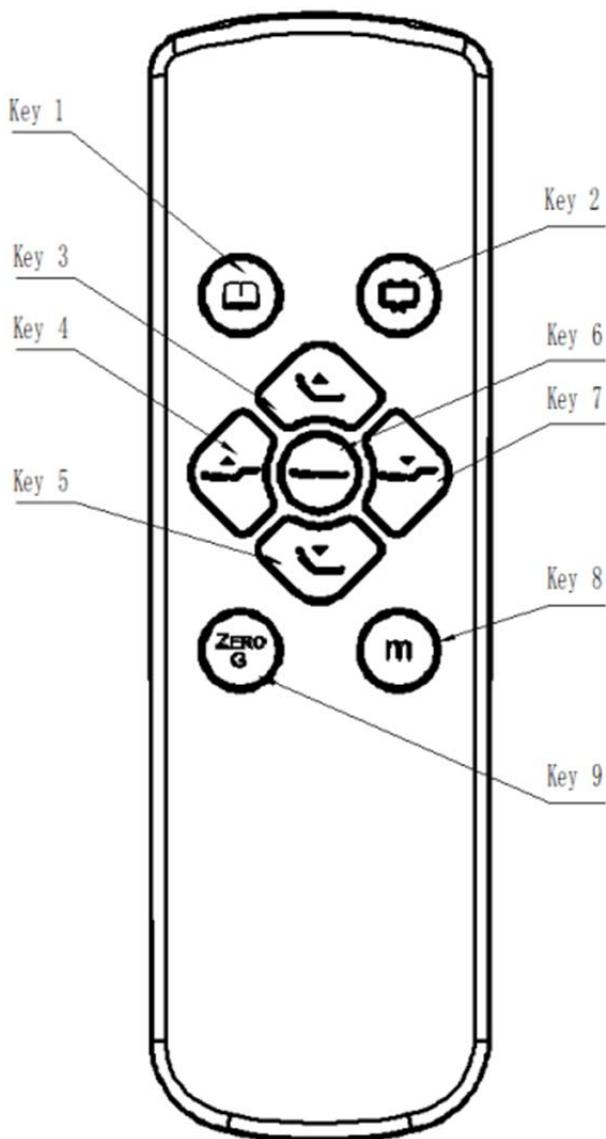
Key 1: Short press button 1, and the fader will run to a fixed position (Book mode) to stop; long press button 1, after 3 seconds, the current position will be memorized (overwrite the previous memory), the backlight will flash 3 times quickly, and the control box will beep
