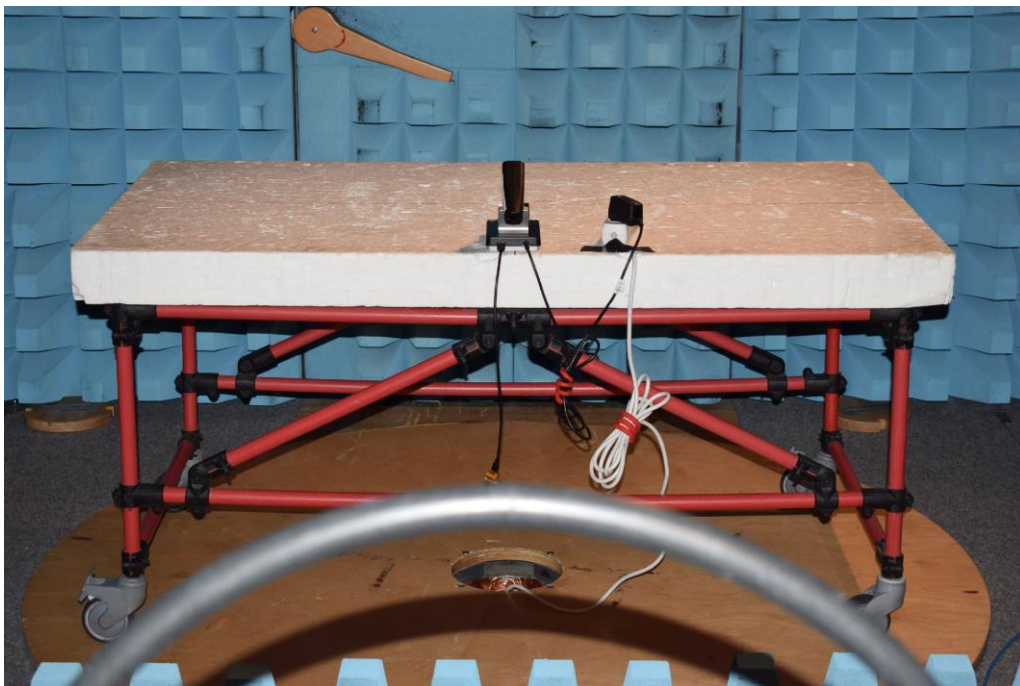
Picture 4: CDC, radiated emission test 9 kHz -30 MHz - Charging (rear view)
