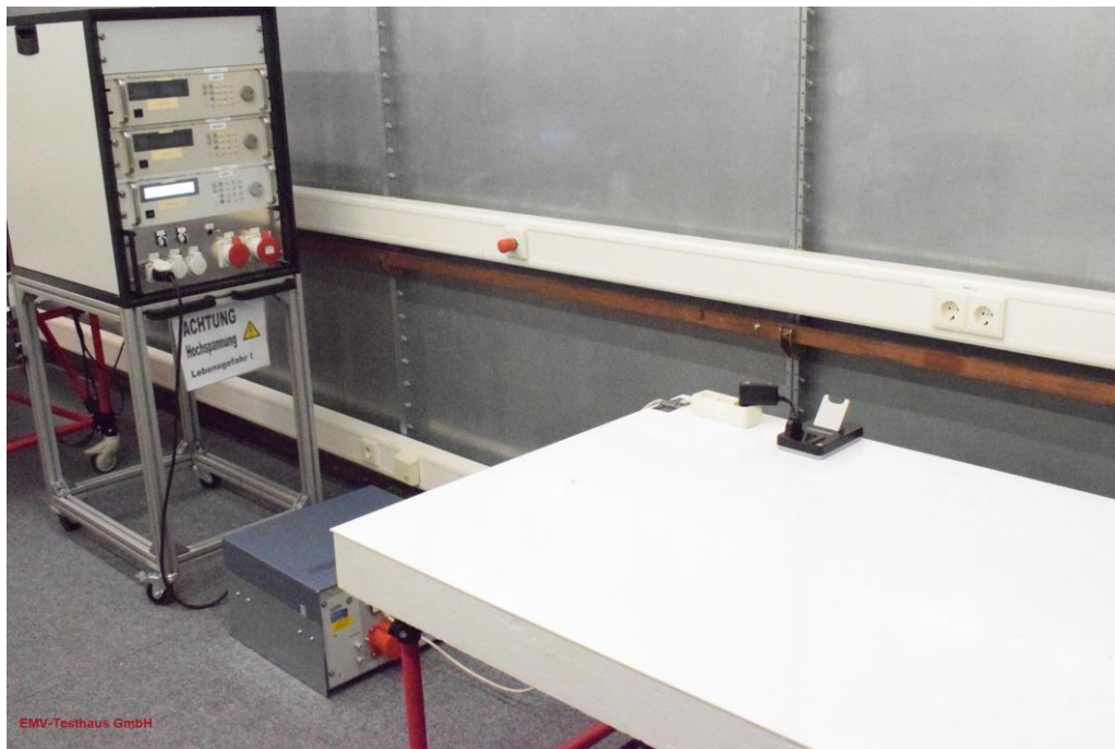
Picture 9: AC power line conducted emission – Standby (front view)
