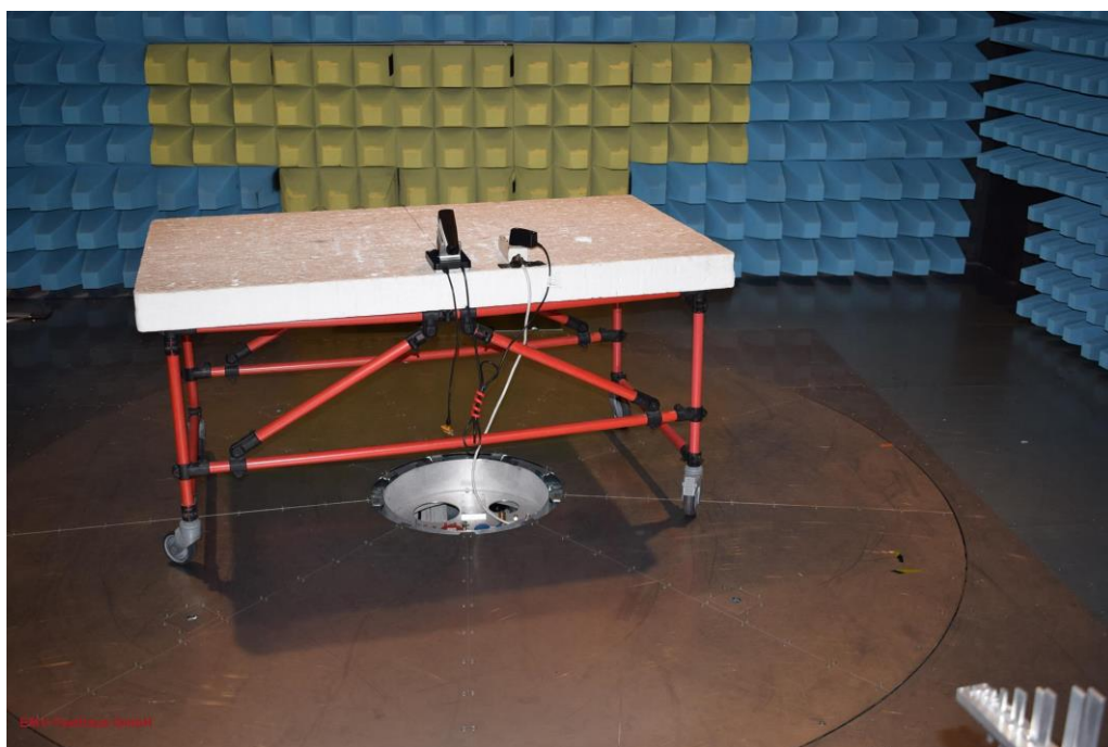
Picture 8: SAC, radiated emission test 30 MHz – 1 GHz – Charging (rear view)
