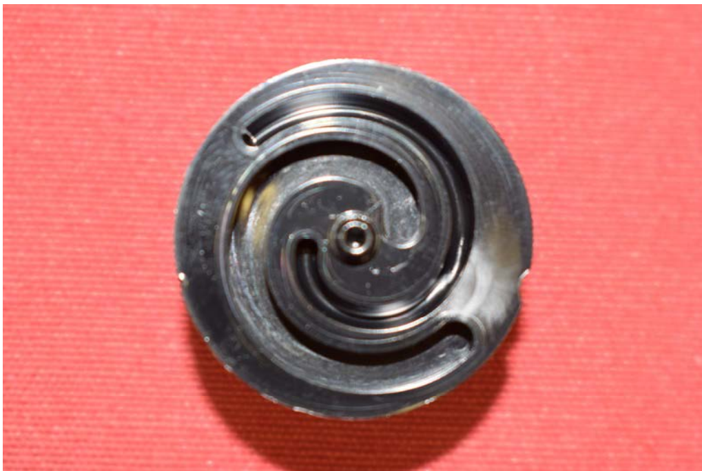
Picture 18: Peripheral device power receiver – focus gear, bottom side
