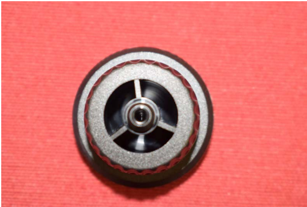
Picture 17: Peripheral device power receiver – focus gear, top side
