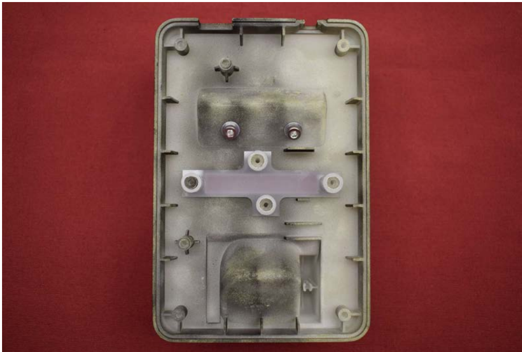
Picture 3: EUT power transmitter – open, bottom side, without PCB
