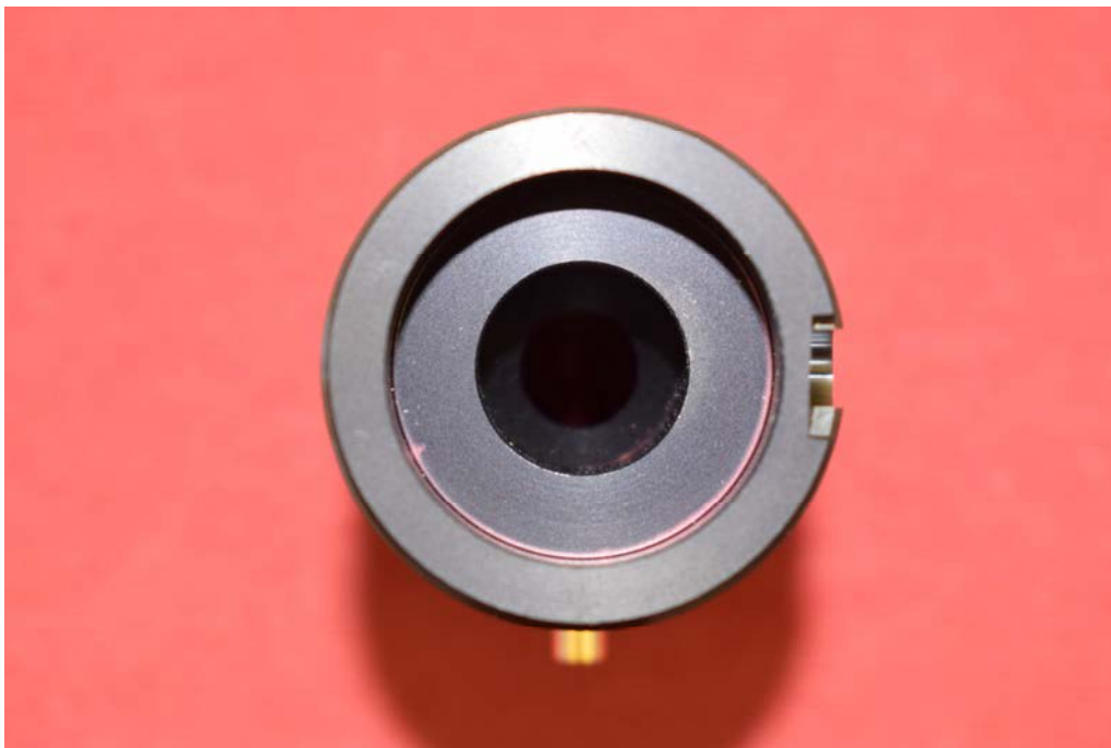
Picture 16: Peripheral device power receiver - magnifying lens, bottom side
