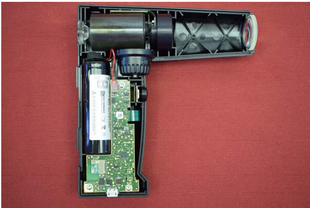
Picture 6: Peripheral device power receiver – open, top side
