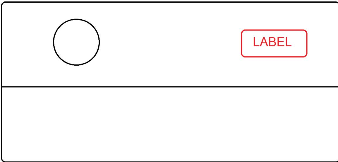
The device label with FCC ID shall be located in the upper right hand corner of the device. The label is affixed to the inner front housing, under the cover.
