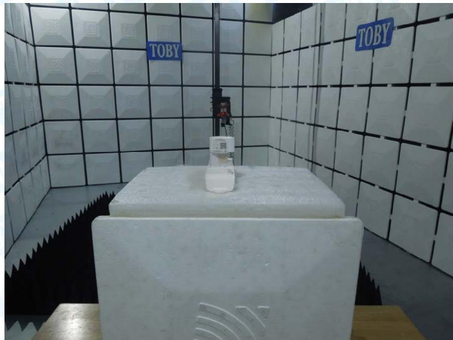
**Photo of Setup for Conducted Emission**
