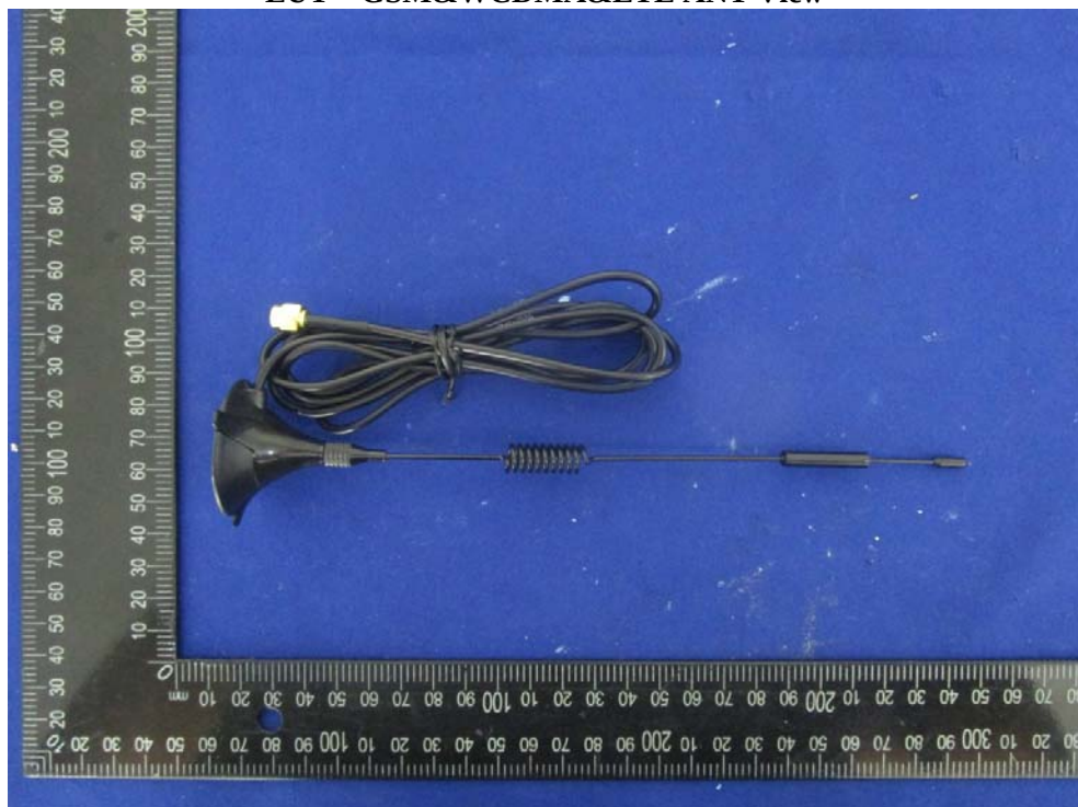
EUT – GSM&WCDMA&LTE ANT View
