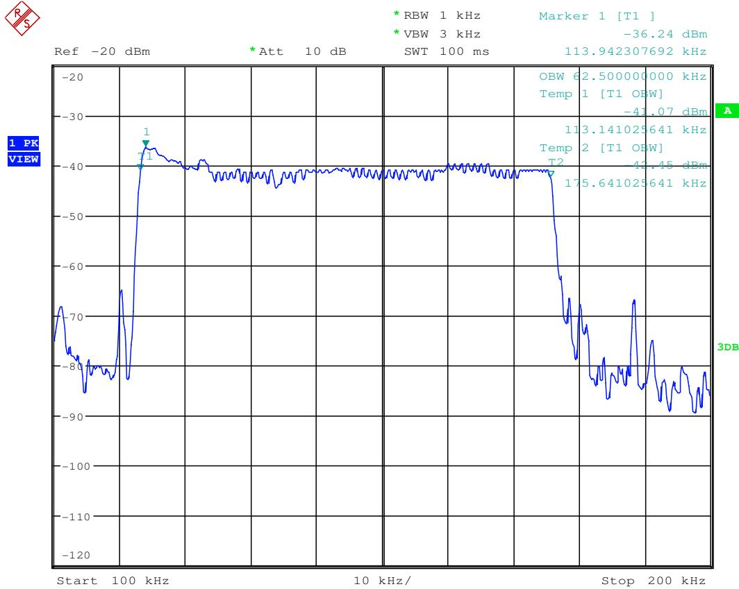
According the test data above, the fundamental wave is not fall in the restricted band 90kHz-110kHz, the field strength also meet the 15.209 requirement, refer to Radiated Emissions (9kHz-30MHz).
