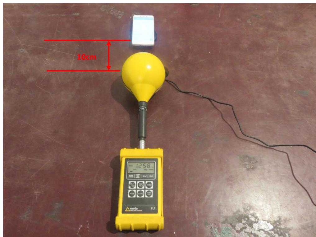
DUT – measurement position D – right side with 10 cm distance charging smartphone (SAMSUNG Galaxy S7)
