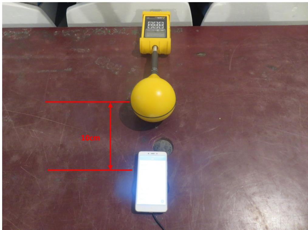
DUT – measurement position B – left side with 10 cm distance charging smartphone (SAMSUNG Galaxy S7)
