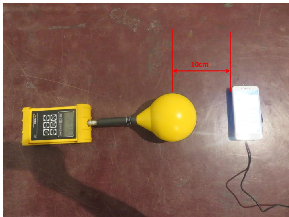
DUT – measurement position C – bottom side with 10 cm distance charging smartphone (SAMSUNG Galaxy S7)
