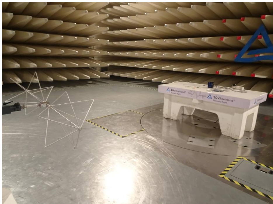
Test setup Frequency Range 30MHz-200MHz Biconical Antenna
