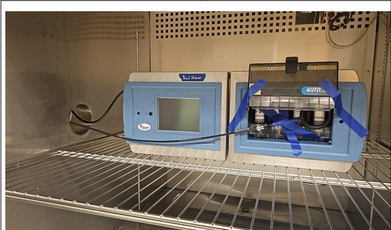
CONDUCTED EUT OBW & FREQUENCY STABILITY SETUP
