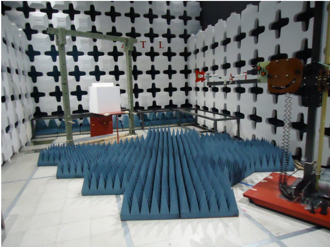
Figure 3.2 - Test Facility (Setup for 1GHz - 18GHz)
