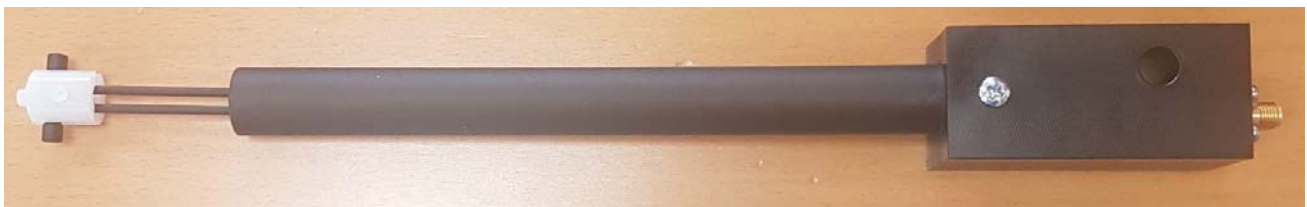
Figure 1 – MVG COMOSAR Validation Dipole
