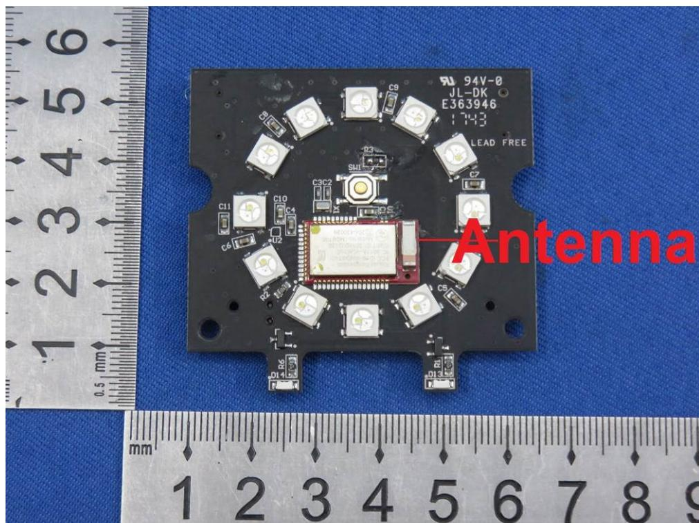
The antenna is integrated on the main PCB and no consideration of replacement. The best case gain of the antenna is 0.5 dBi.
