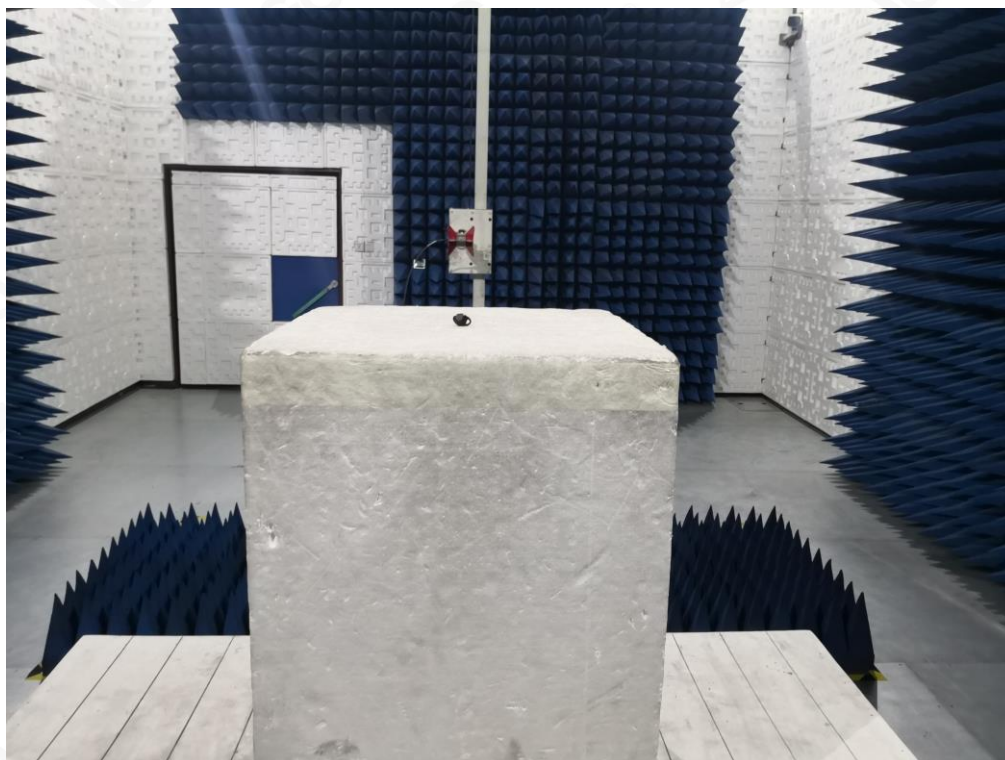
RADIATED EMISSION TEST SETUP ABOVE 1GHZ
