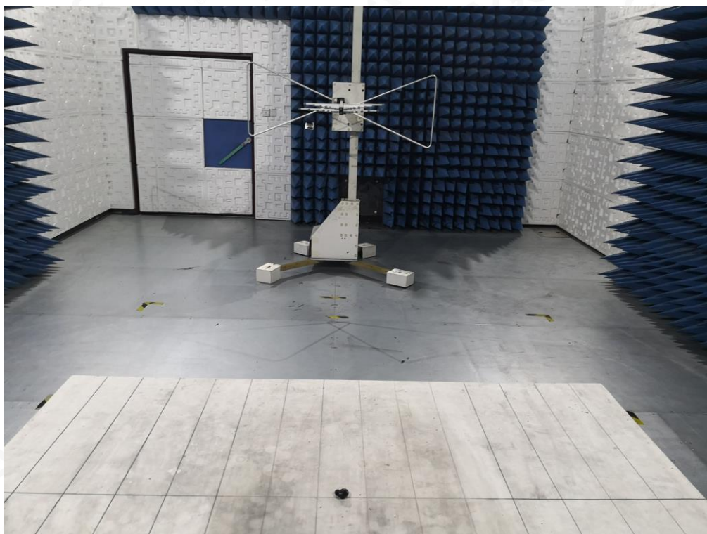
RADIATED EMISSION TEST SETUP ABOVE 1GHZ
