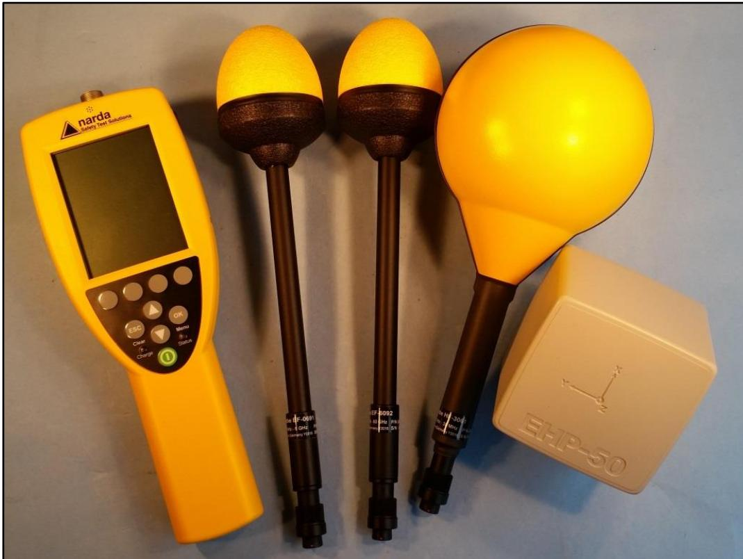
A state of the art Broadband Electromagnetic Field Test system was used. The probes of the system are fitted with three sensors which measure the field strength of the X, Y and Z plane directions separately. The field strength is calculated by the instrument's processor by summing the squares of the three measured values.
