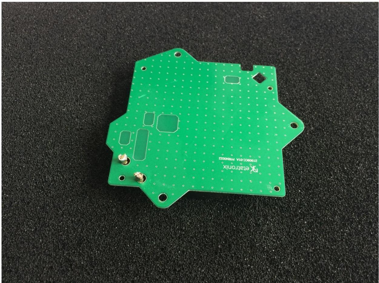
The following picture shows the Top View of the Data Coil:
