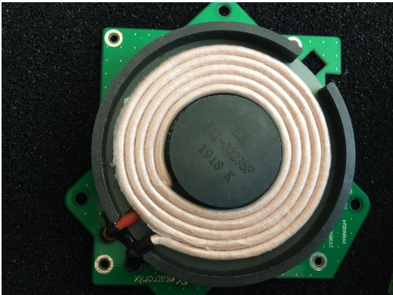
The following picture shows the Bottom View of the Power Coil:
