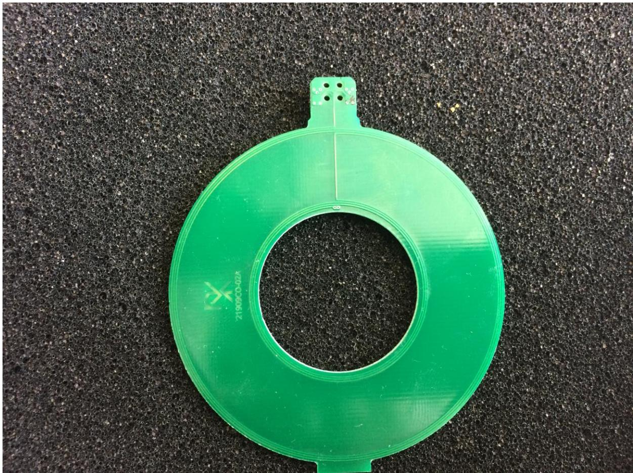
The following picture shows the Bottom View of the Data Coil:
