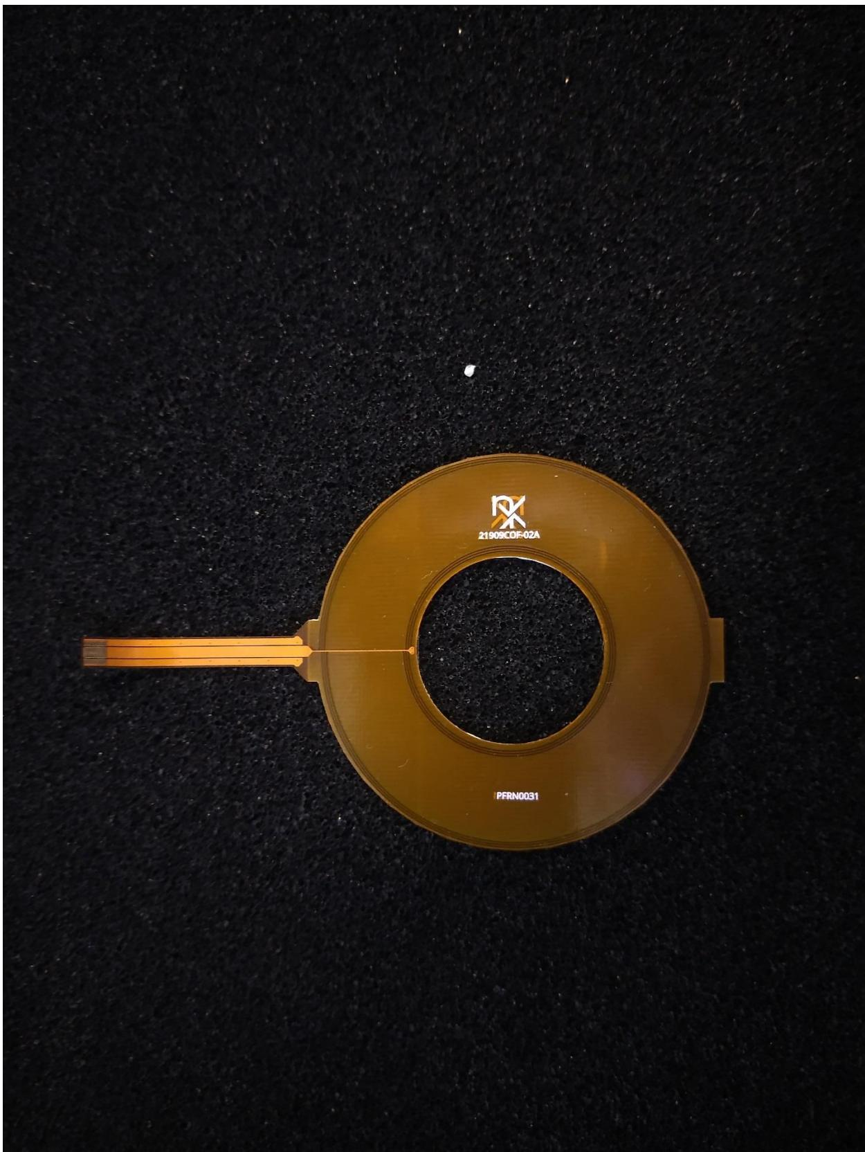
The following picture shows the Bottom View of the Data Coil:
