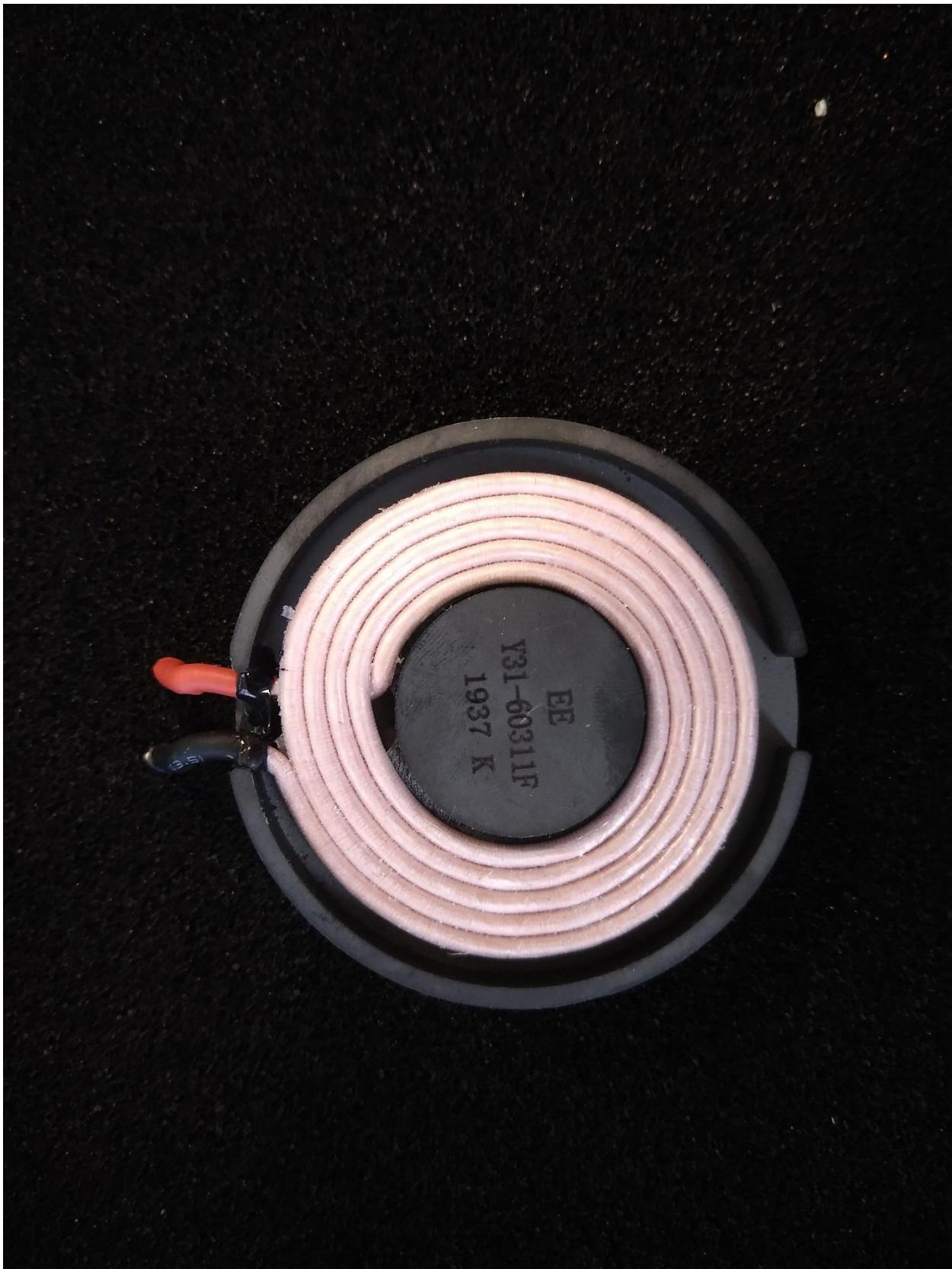
The following picture shows the Bottom View of the Power Coil:
