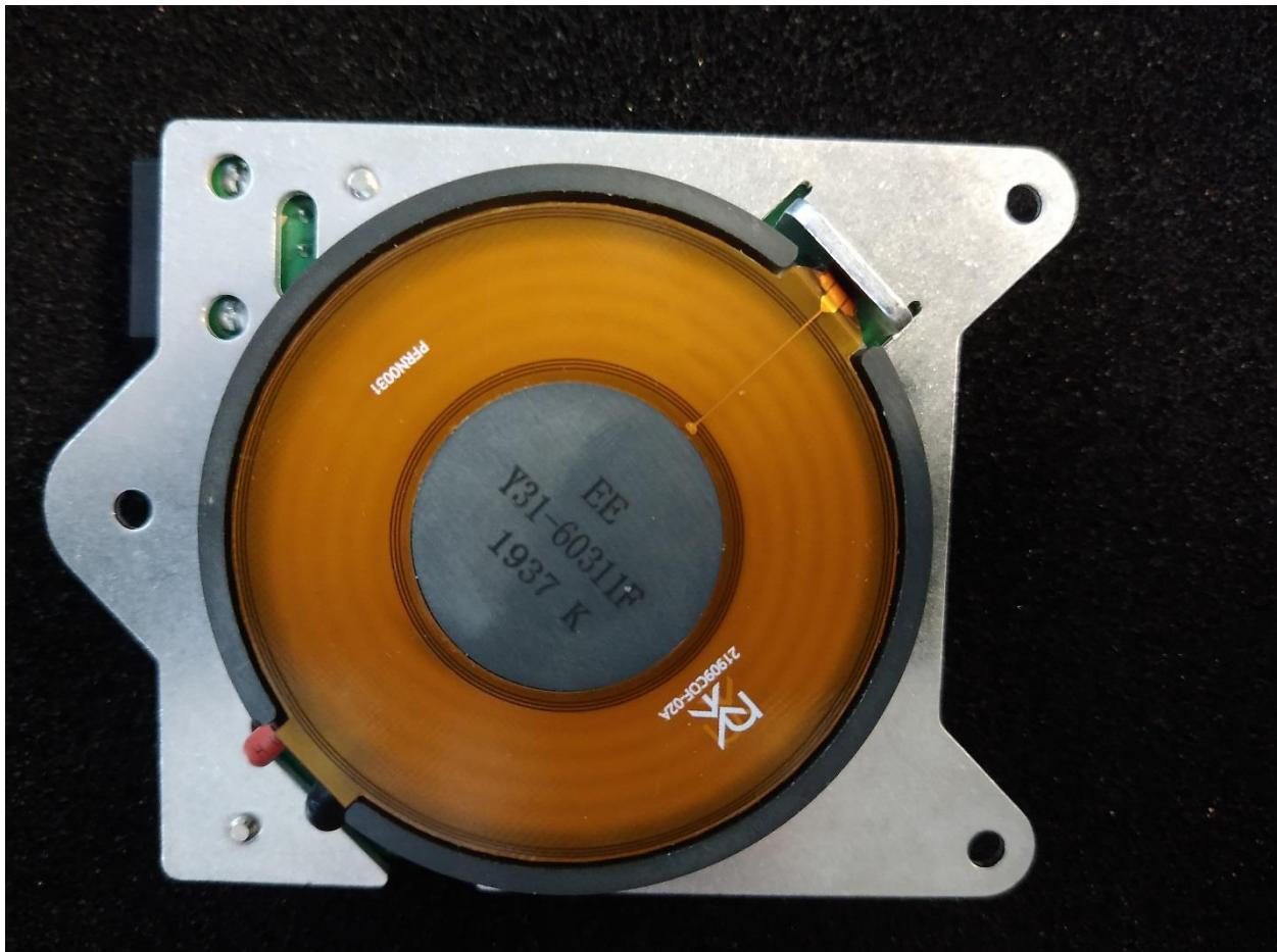
The following picture shows the Top View of the Power Coil:
