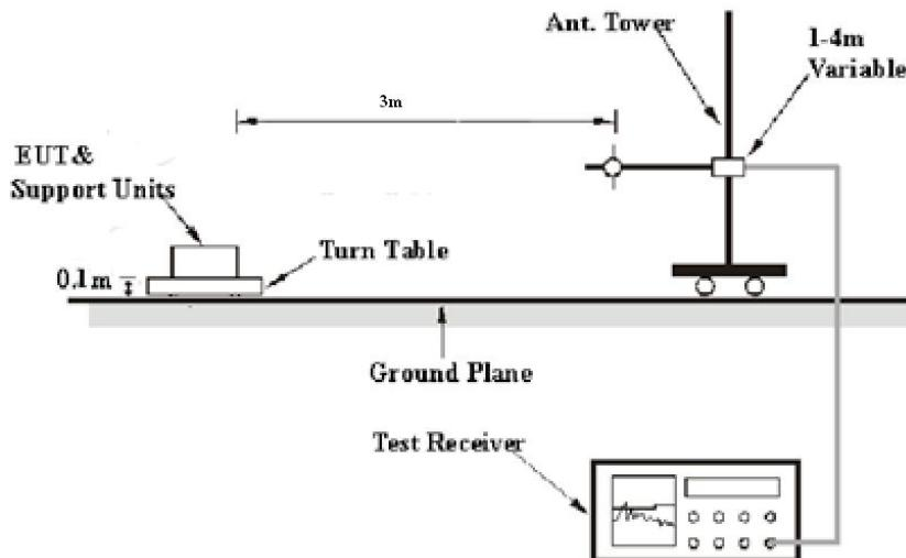
The radiated emission tests were performed in the 3-meter chamber test site, using the setup accordance with the ANSI C63.10-2013. The specification used was the FCC Part Subpart C limits.
