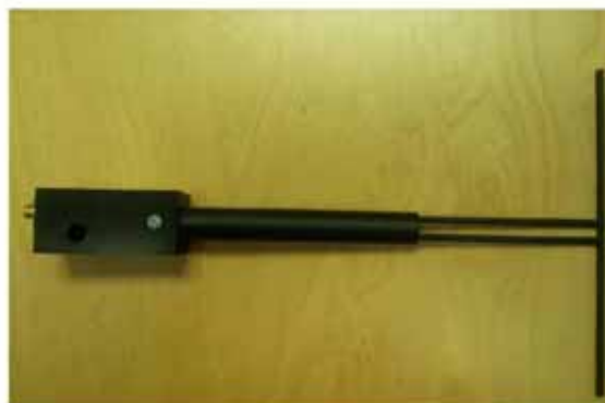
Figure 1 – MVG COMOSAR Validation Dipole
