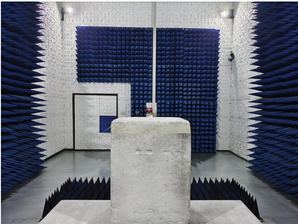
RADIATED EMISSION TEST SETUP ABOVE 1GHz
