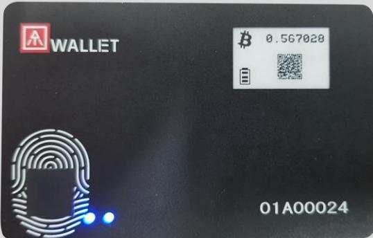
AT.Wallet is an USB/BLE **fingerprint Hardware Wallet** for cryptocurrency transaction (for example Bitcoin, Bitcoin cash, Ethereum, ....) through BLE or USB app; and comparing with hot wallet (app, web, ...), AT.Wallet protects private keys inside SE and never leave it, plus fingerprint identification users to avoid hackers.
