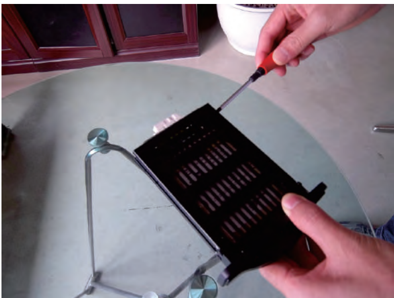
Picture 12: HDD enclosure installation image 1
