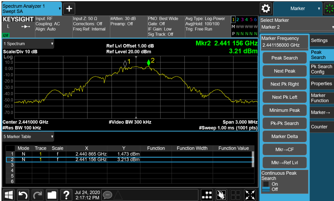
Figure 24: Hopping Frequency Separation, Hopping Mode, GFSK
