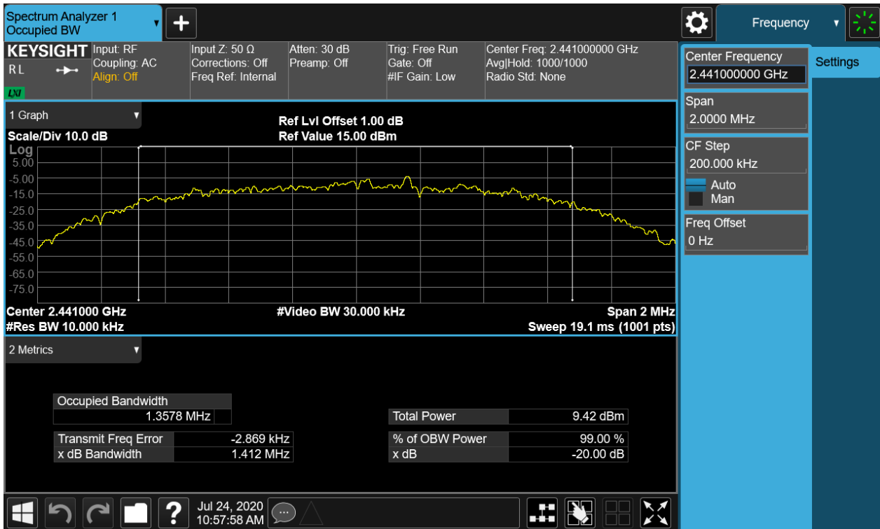
Figure 14: 20dB Bandwidth and 99% Bandwidth, 2441MHz, 8-DPSK
