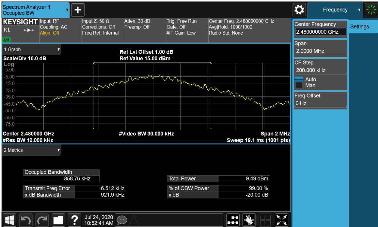
Figure 12: 20dB Bandwidth and 99% Bandwidth, 2480MHz, GFSK
