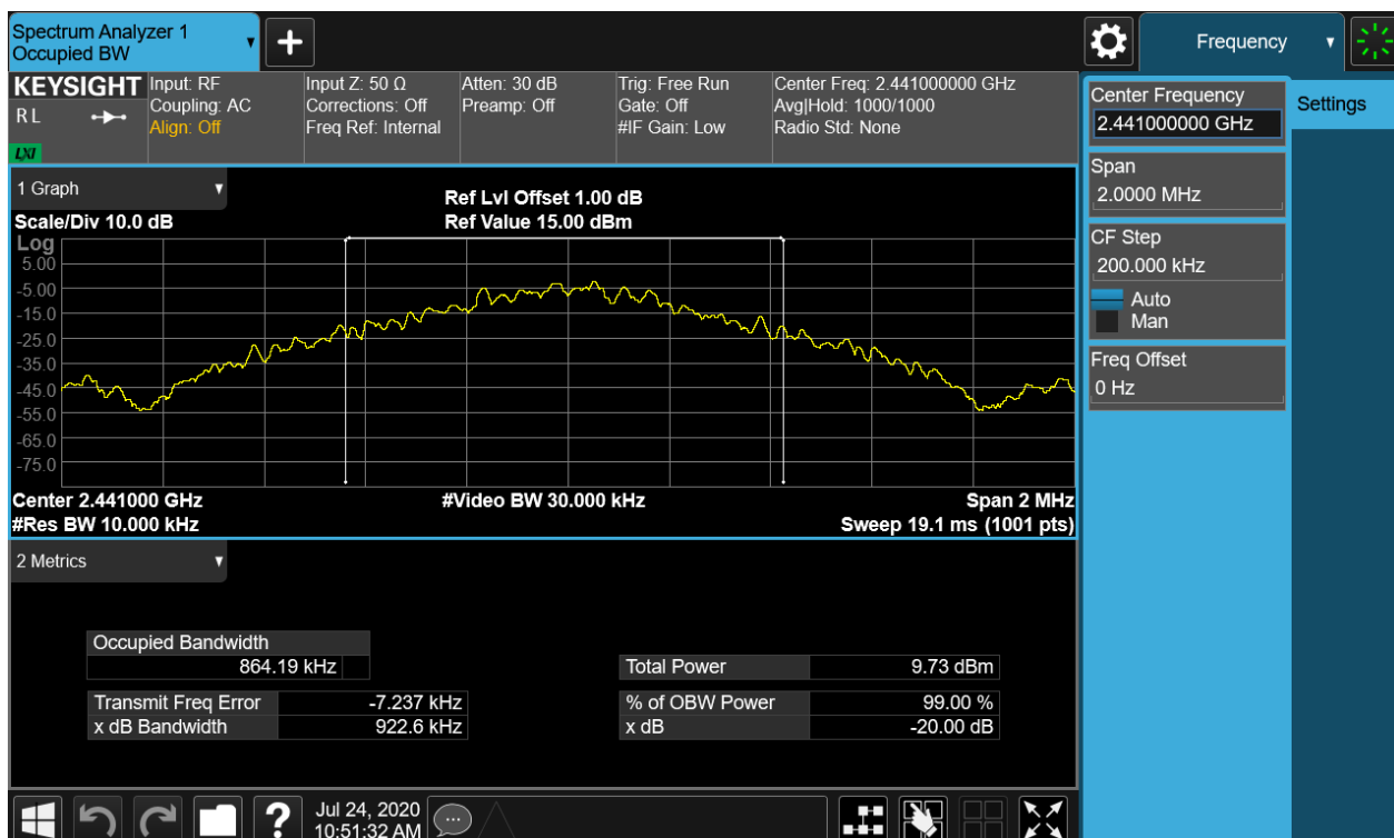
Figure 11: 20dB Bandwidth and 99% Bandwidth, 2441MHz, GFSK
