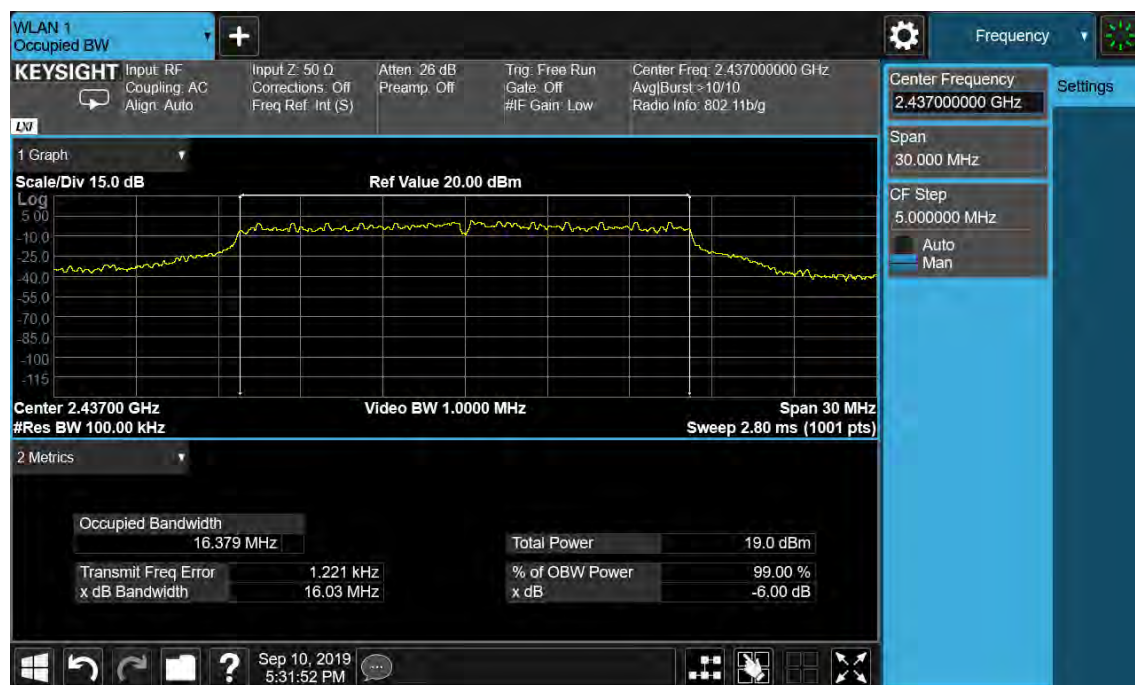
Figure 5: 6dB Bandwidth and 99% Bandwidth, 802.11g, 2437MHz
