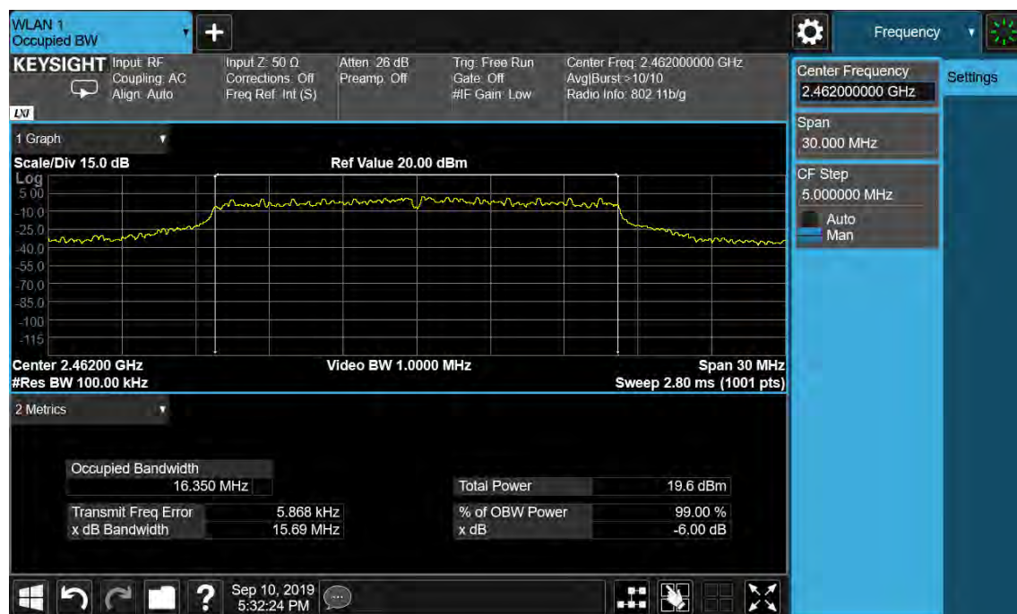
Figure 6: 6dB Bandwidth and 99% Bandwidth, 802.11g, 2462MHz
