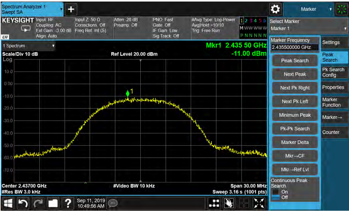
Figure 14: Power Spectral Density, 802.11b, 2437MHz
