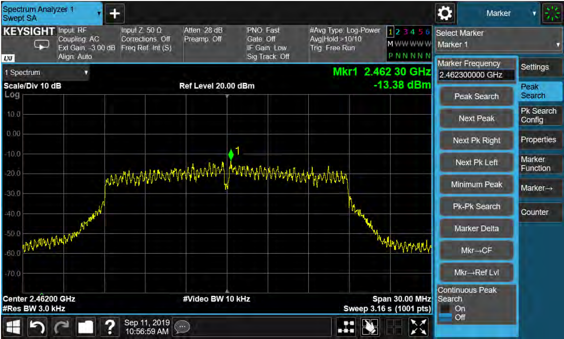
Figure 21: Power Spectral Density, 802.11n(HT20), 2462MHz
