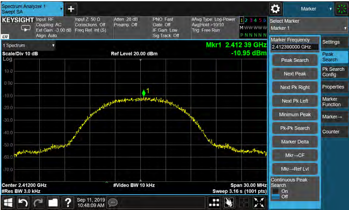
Figure 13: Power Spectral Density, 802.11b, 2412MHz
