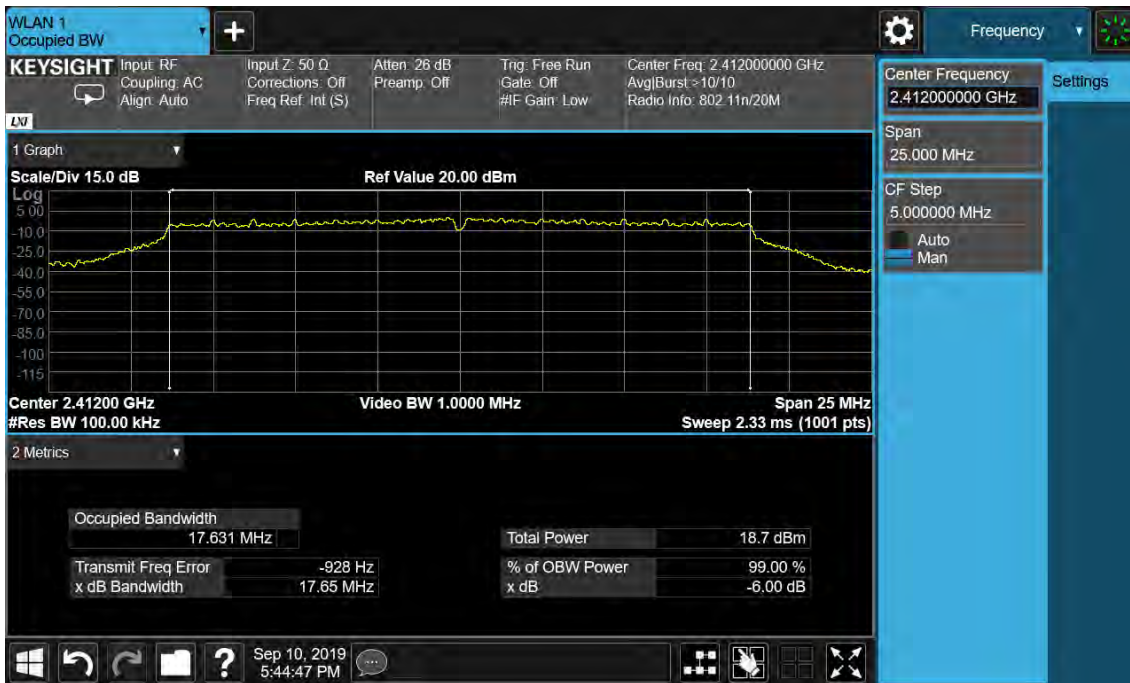
Figure 7: 6dB Bandwidth and 99% Bandwidth, 802.11n(HT20), 2412MHz
