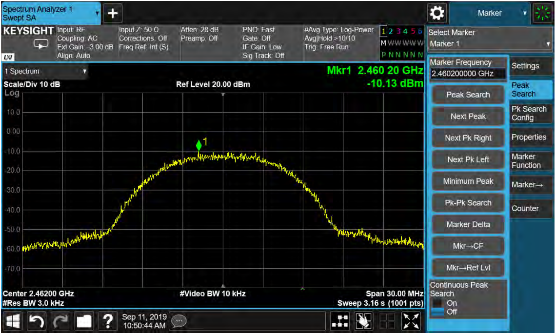
Figure 15: Power Spectral Density, 802.11b, 2462MHz
