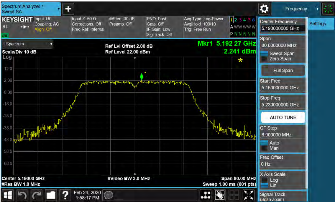
Figure 52: Power Spectral Density, 802.11n(HT40), 5190MHz
