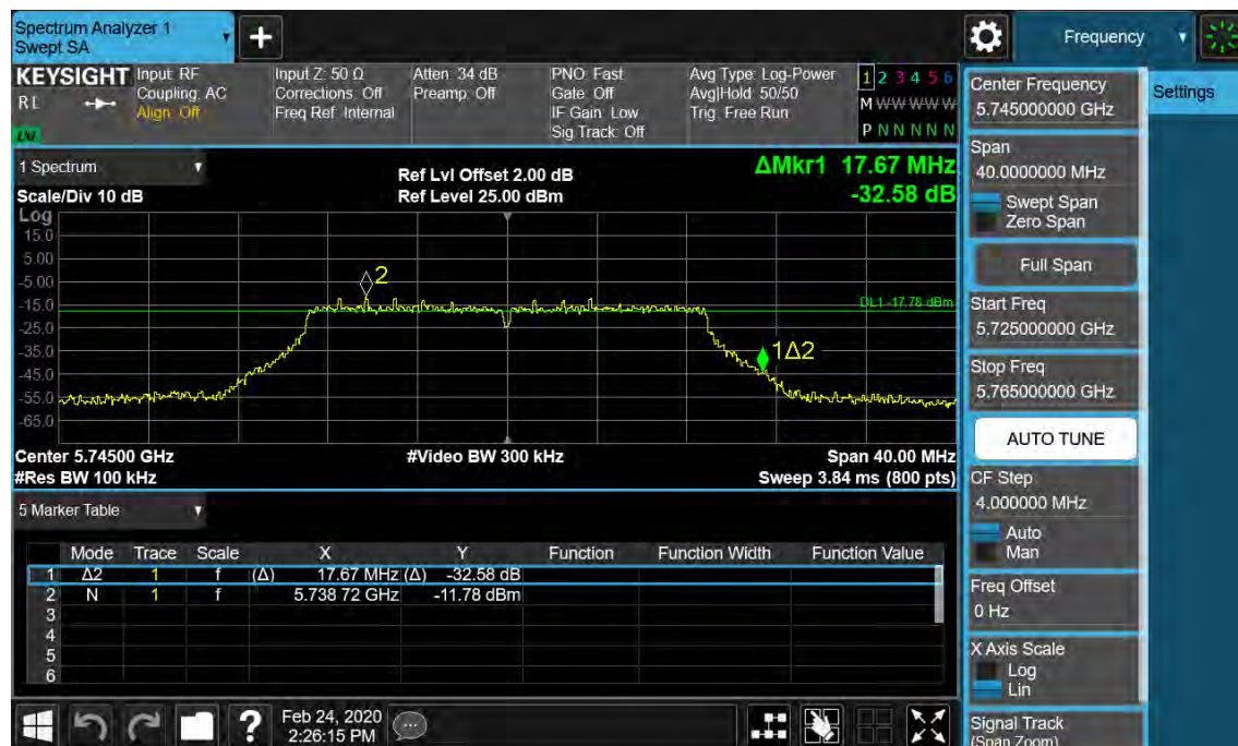
Figure 32: 6dB Bandwidth, 802.11n(HT20), 5745MHz
