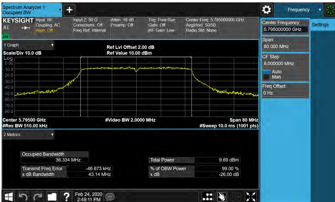
Figure 28: 26dB Bandwidth and 99% Bandwidth, 802.11ac(VHT80), 5775MHz
