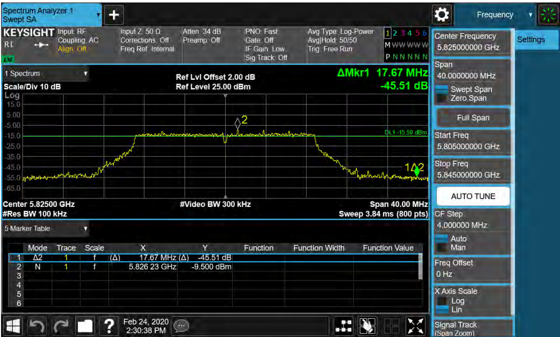
Figure 34: 6dB Bandwidth, 802.11n(HT20), 5825MHz
