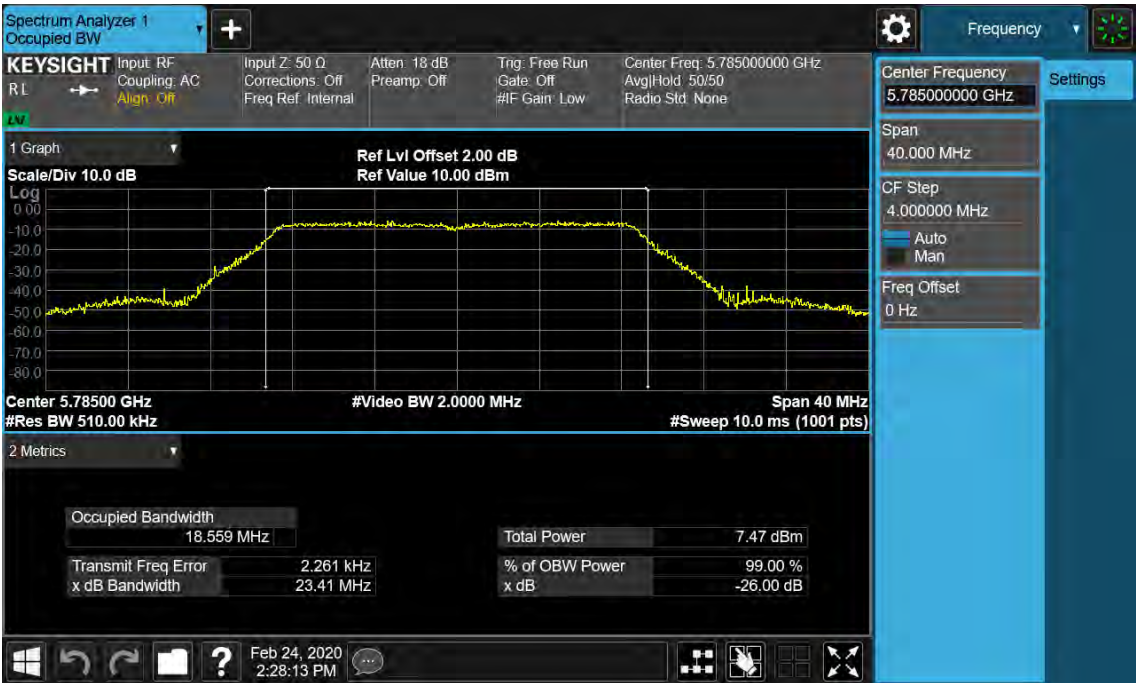
Figure 20: 26dB Bandwidth and 99% Bandwidth, 802.11n(HT20), 5825MHz
