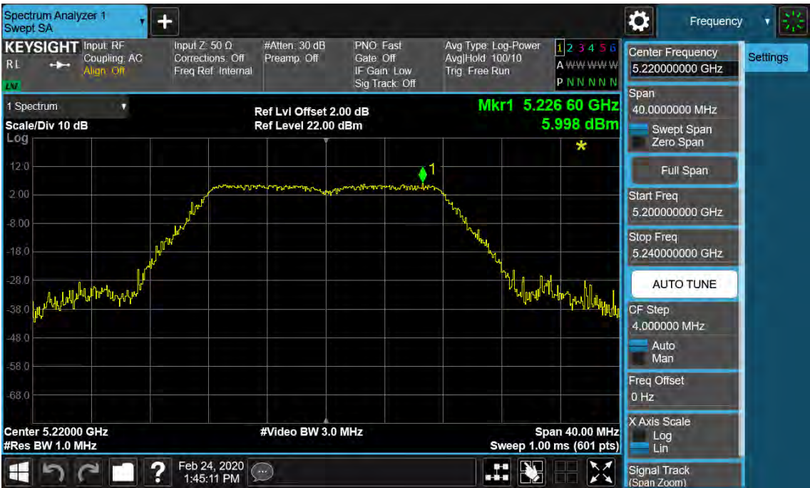
Figure 44: Power Spectral Density, 802.11a, 5220MHz
