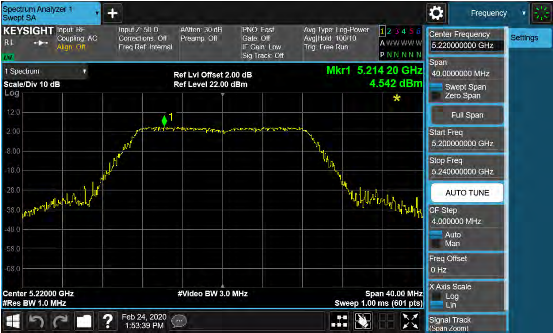
Figure 47: Power Spectral Density, 802.11n(HT20), 5220MHz
