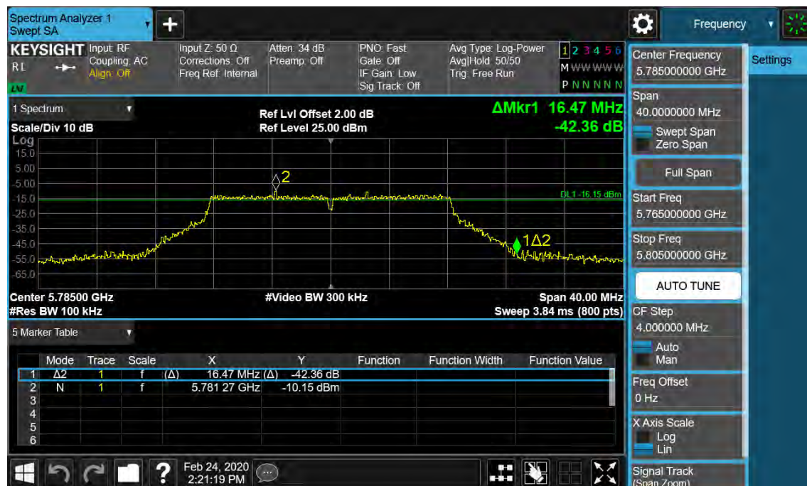
Figure 30: 6dB Bandwidth, 802.11a, 5785MHz
