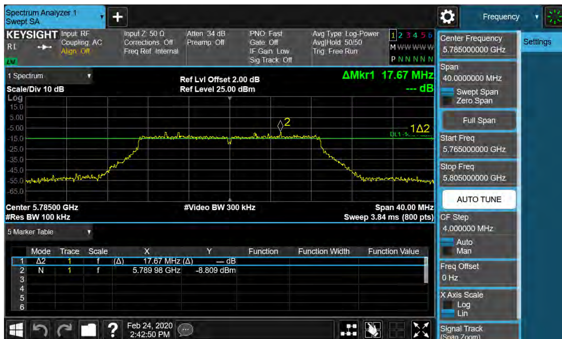
Figure 36: 6dB Bandwidth, 802.11ac(VHT20), 5785MHz
