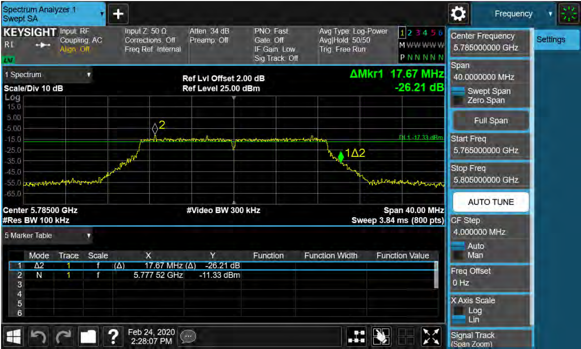
Figure 33: 6dB Bandwidth, 802.11n(HT20), 5785MHz
