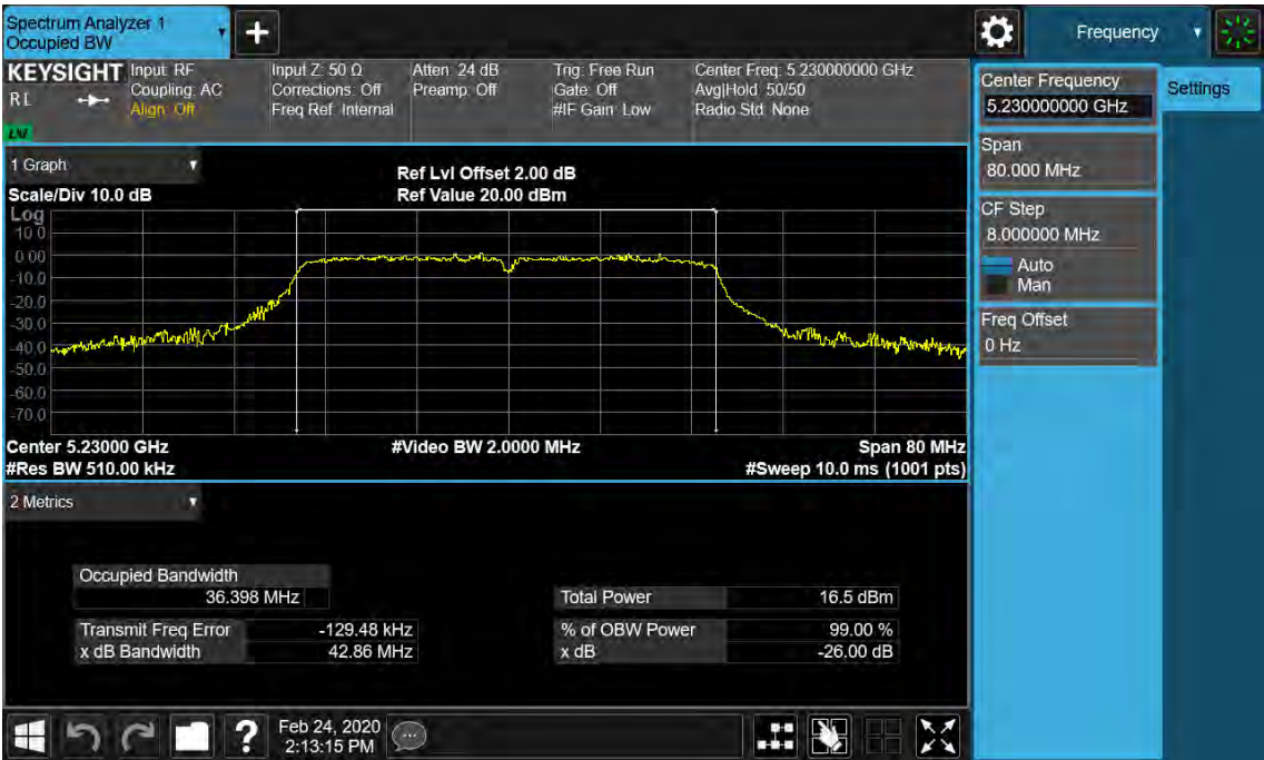
Figure 14: 26dB Bandwidth and 99% Bandwidth, 802.11ac(VHT80), 5210MHz
