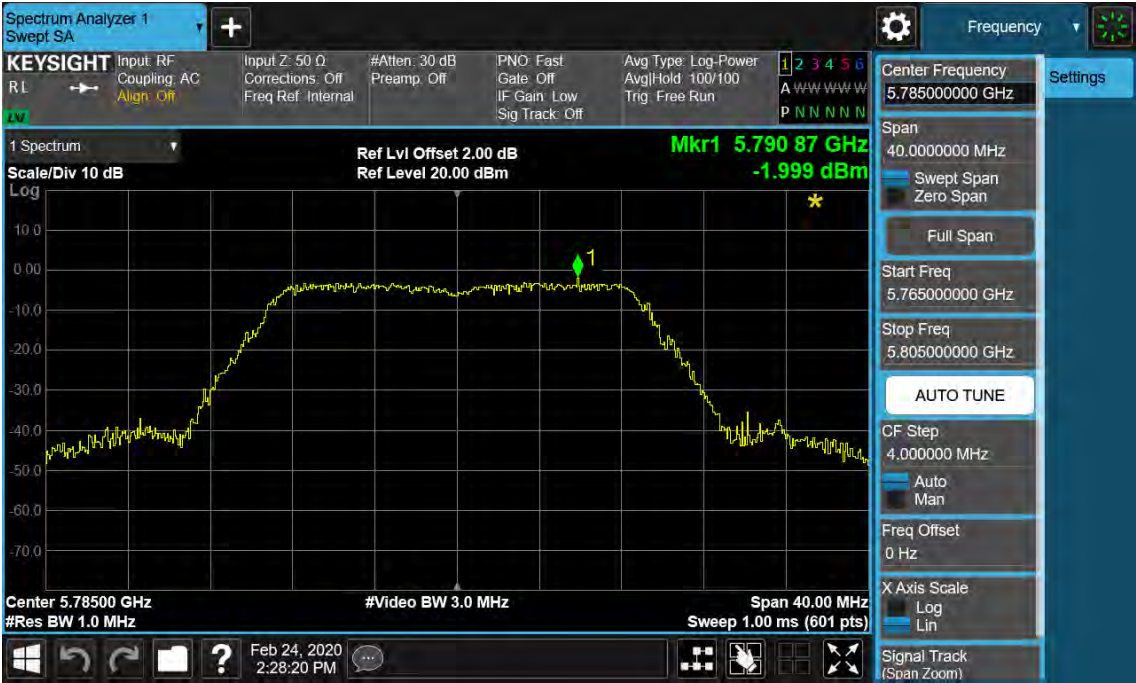
Figure 61: Power Spectral Density, 802.11n(HT20), 5785MHz
