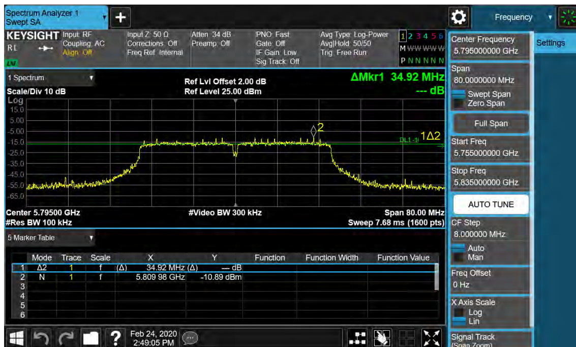
Figure 41: 6dB Bandwidth, 802.11ac(VHT40), 5785MHz
