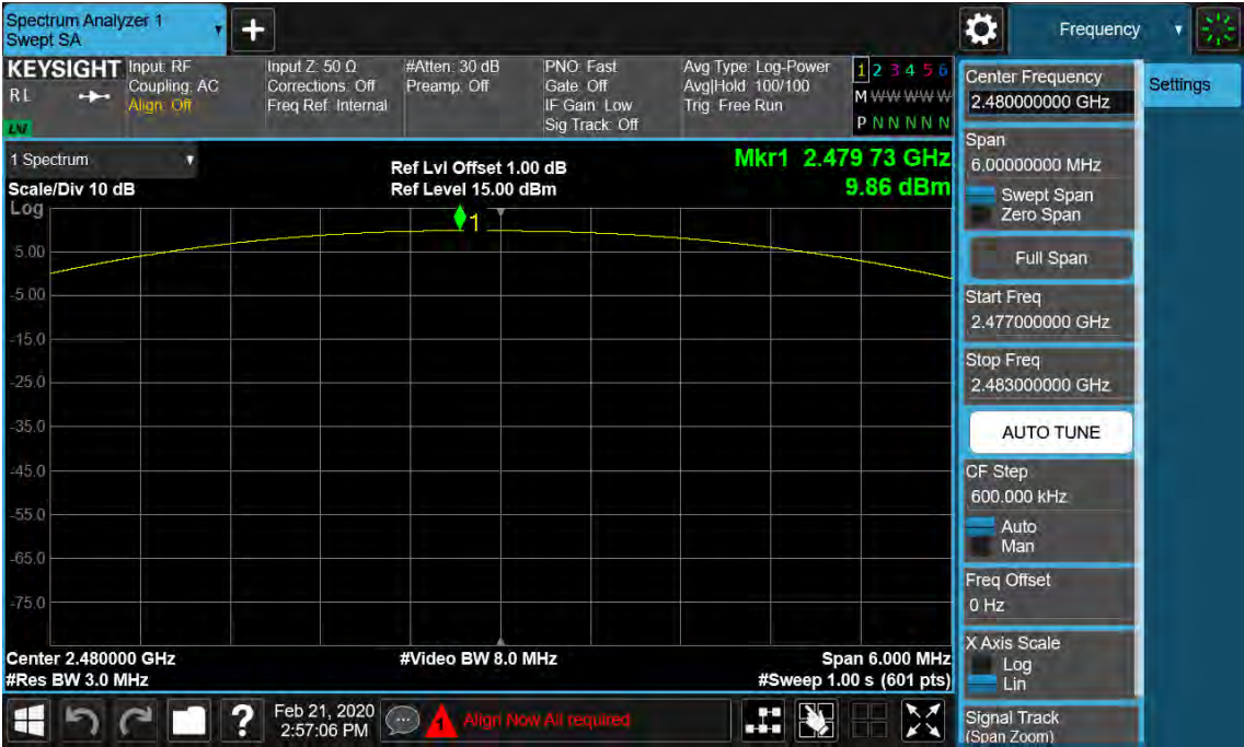
Figure 3: Maximum Conducted Output Power, 2480MHz, GFSK
