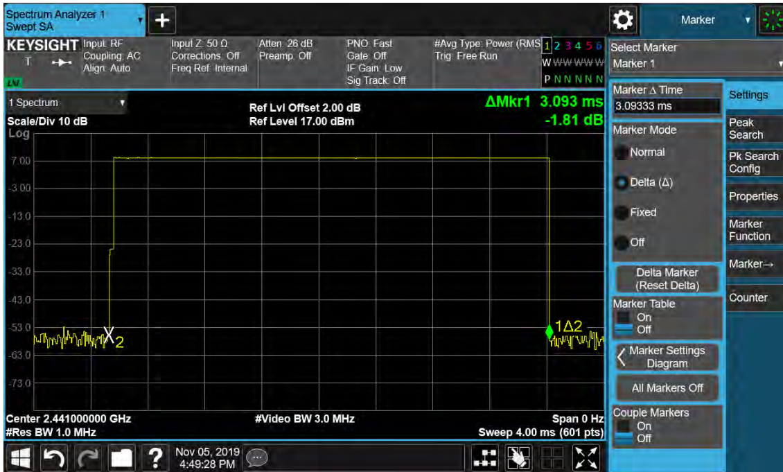
Figure 45: Time of Occupancy, 2441MHz, GFSK DH5
