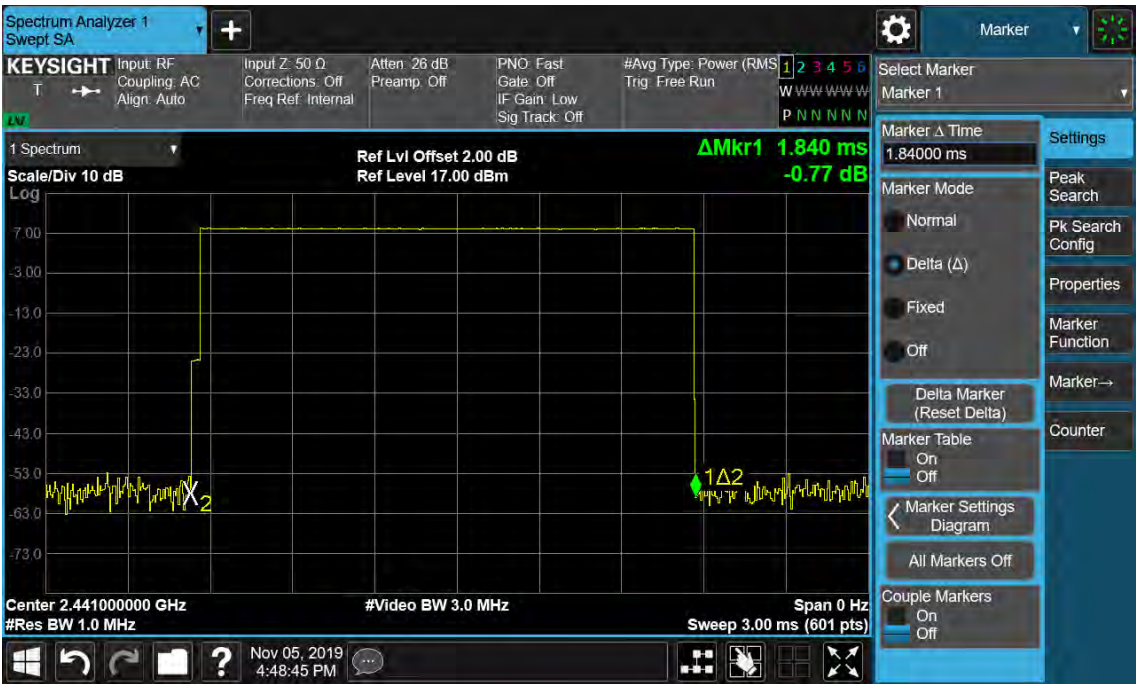
Figure 44: Time of Occupancy, 2441MHz, GFSK DH3
