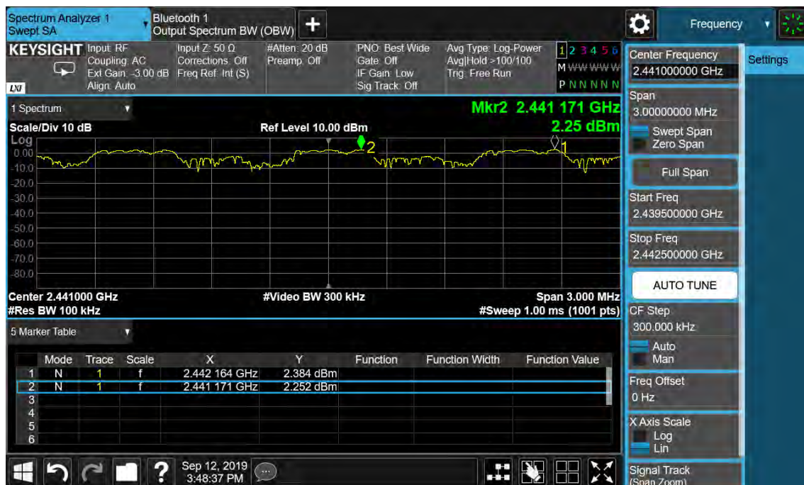
Figure 40: Hopping Frequency Separation, Hopping Mode, 8DPSK
