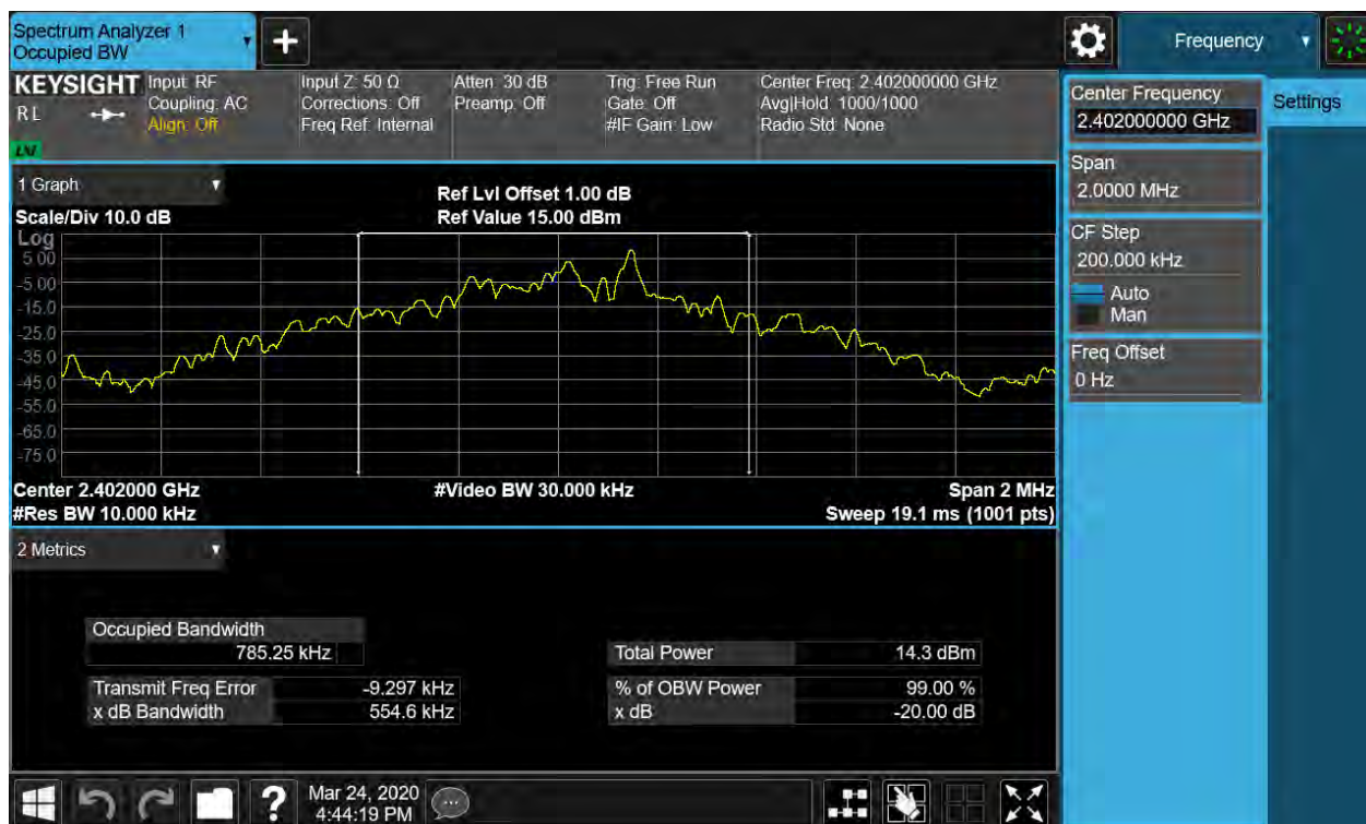
Figure 10: 20dB Bandwidth and 99% Bandwidth, 2402MHz, GFSK
