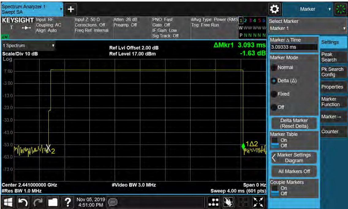
Figure 48: Time of Occupancy, 2441MHz, 8-DPSK DH5
