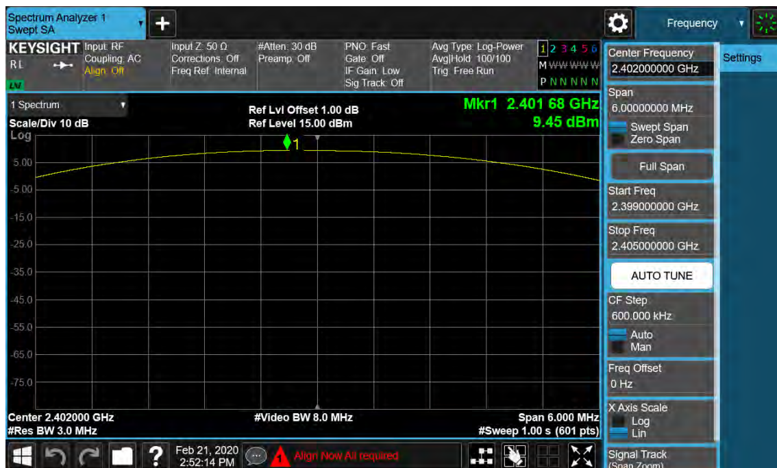
Figure 1: Maximum Conducted Output Power, 2402MHz, GFSK
