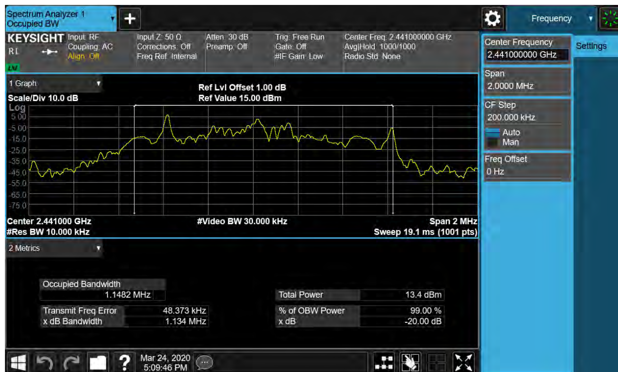
Figure 14: 20dB Bandwidth and 99% Bandwidth, 2441MHz, 8-DPSK
