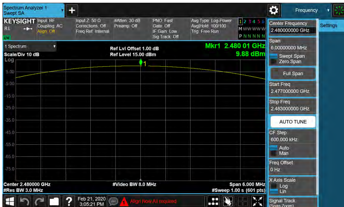
Figure 6: Maximum Conducted Output Power, 2480MHz, \pi/4 -DQPSK
