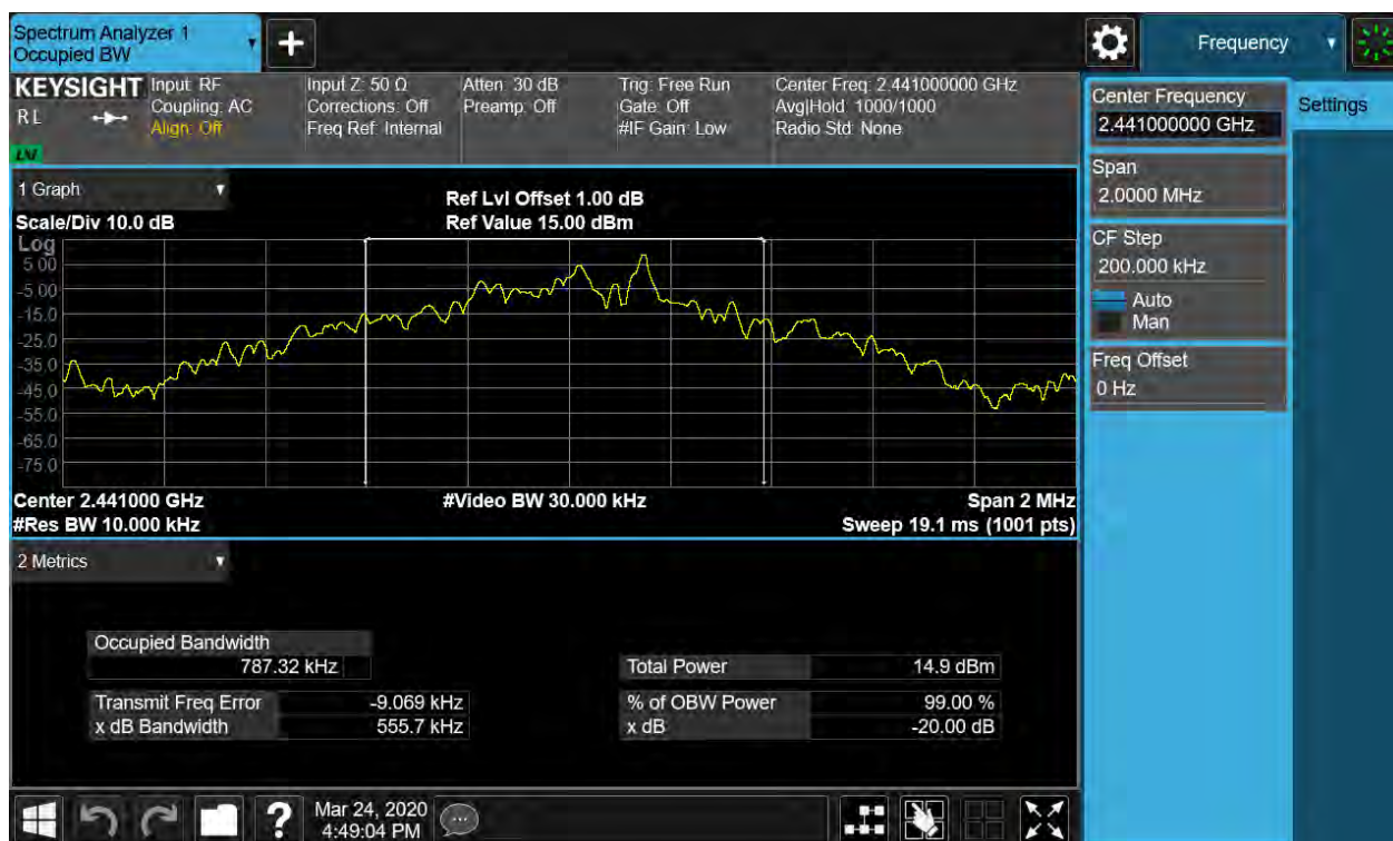
Figure 11: 20dB Bandwidth and 99% Bandwidth, 2441MHz, GFSK
