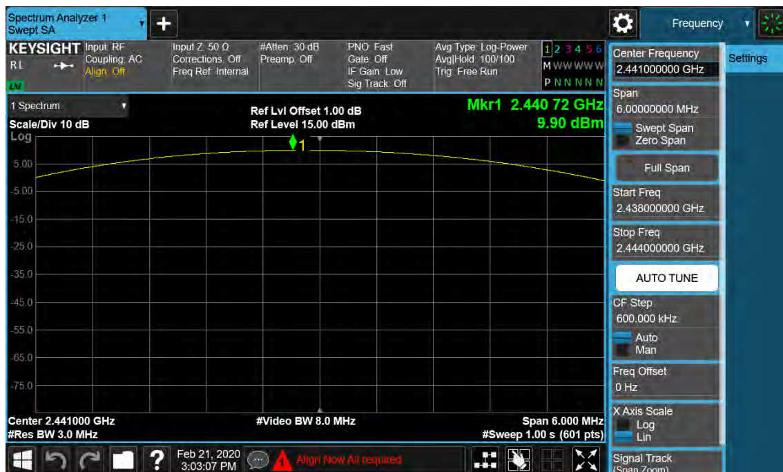
Figure 5: Maximum Conducted Output Power, 2441MHz, \pi/4 -DQPSK
