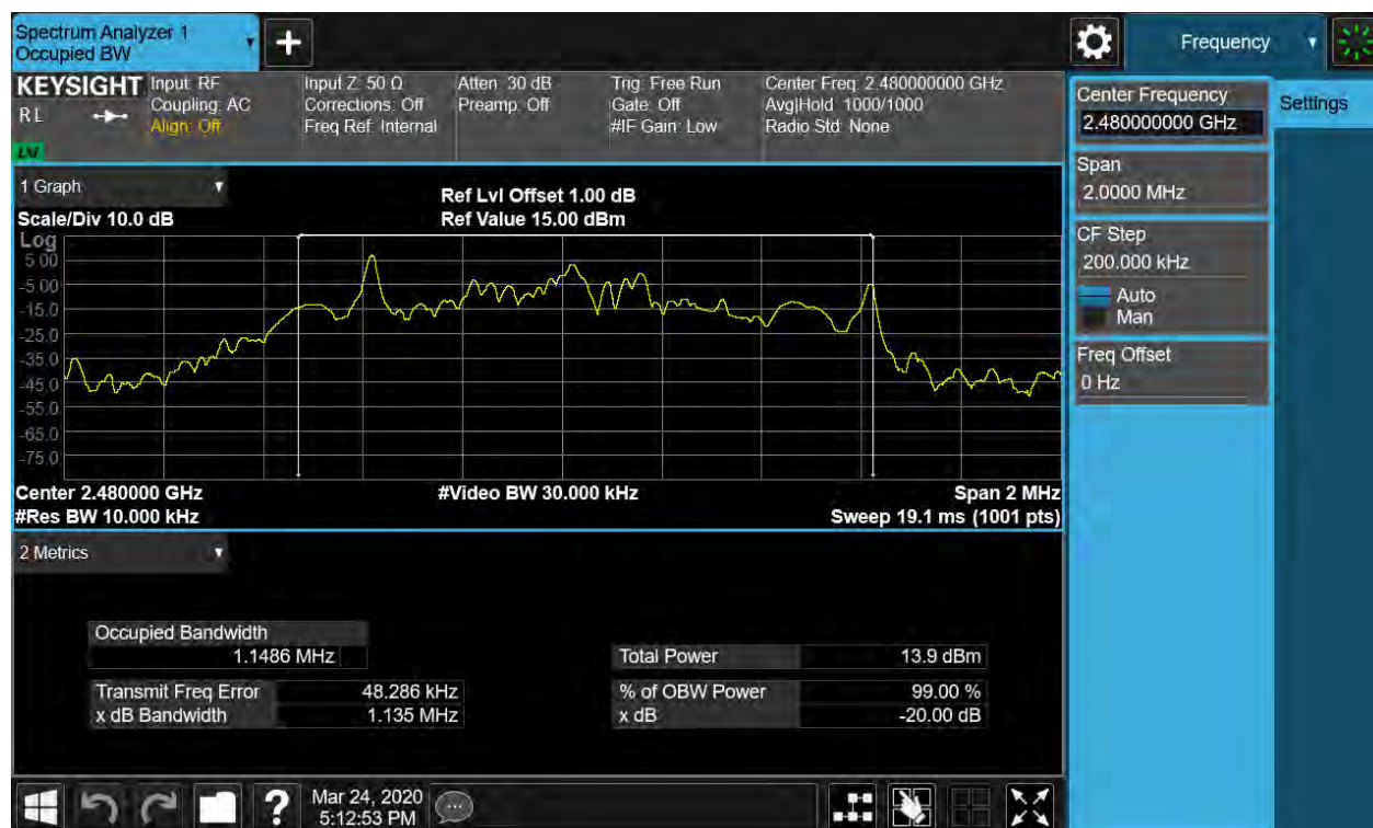
Figure 15: 20dB Bandwidth and 99% Bandwidth, 2480MHz, 8-DPSK
