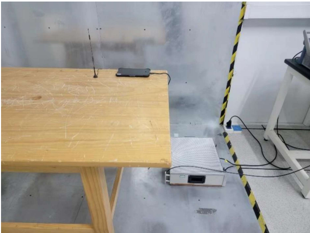
Radiated Emission test set-up for 30M-1GHz, TM1
