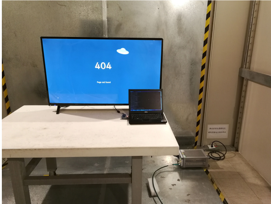
Conducted Emissions (Side View)
