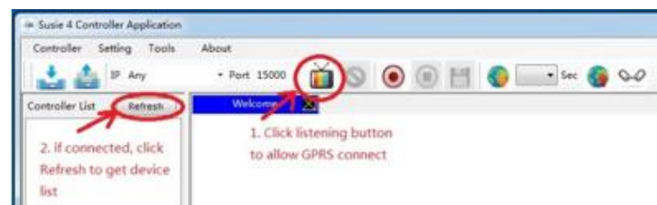
Figure 8: Connecting to Susie IV via GPRS
