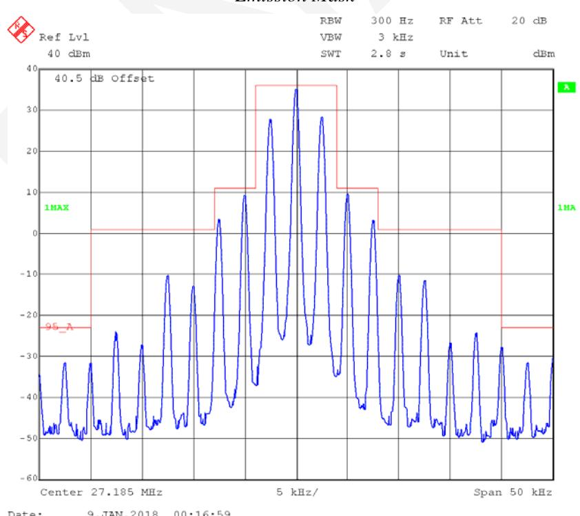
**FCC §2.1053,§95.979 - SPURIOUS EMISSIONS AT ANTENNA TERMINALS****Applicable Standard**
