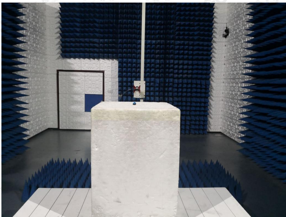
RADIATED EMISSION TEST SETUP ABOVE 1GHZ
