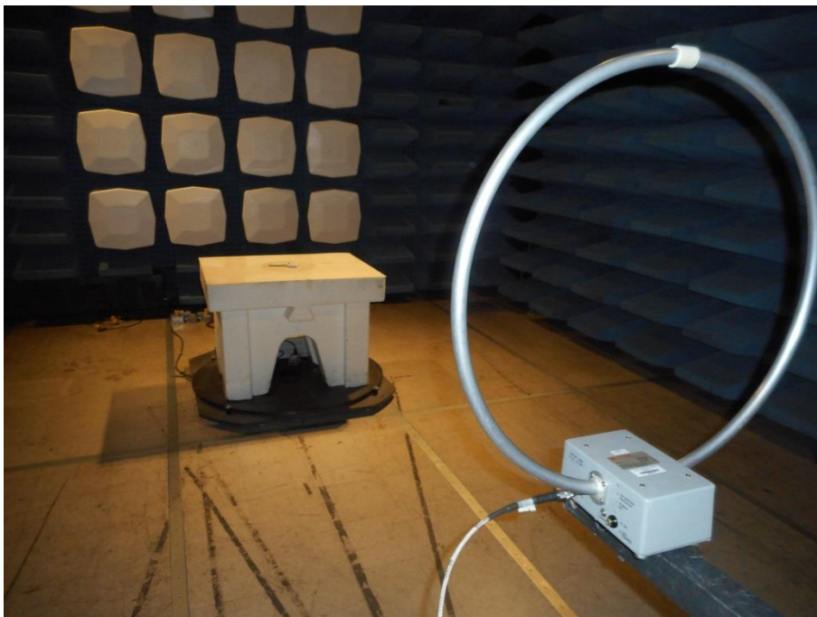
Figure 4: Radiated Emissions performed (Below 30MHz) at the SAC Test Setup
