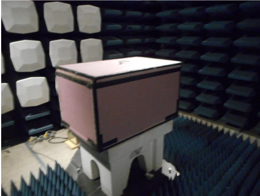
Figure 3: Radiated Emissions SAC Test Setup
