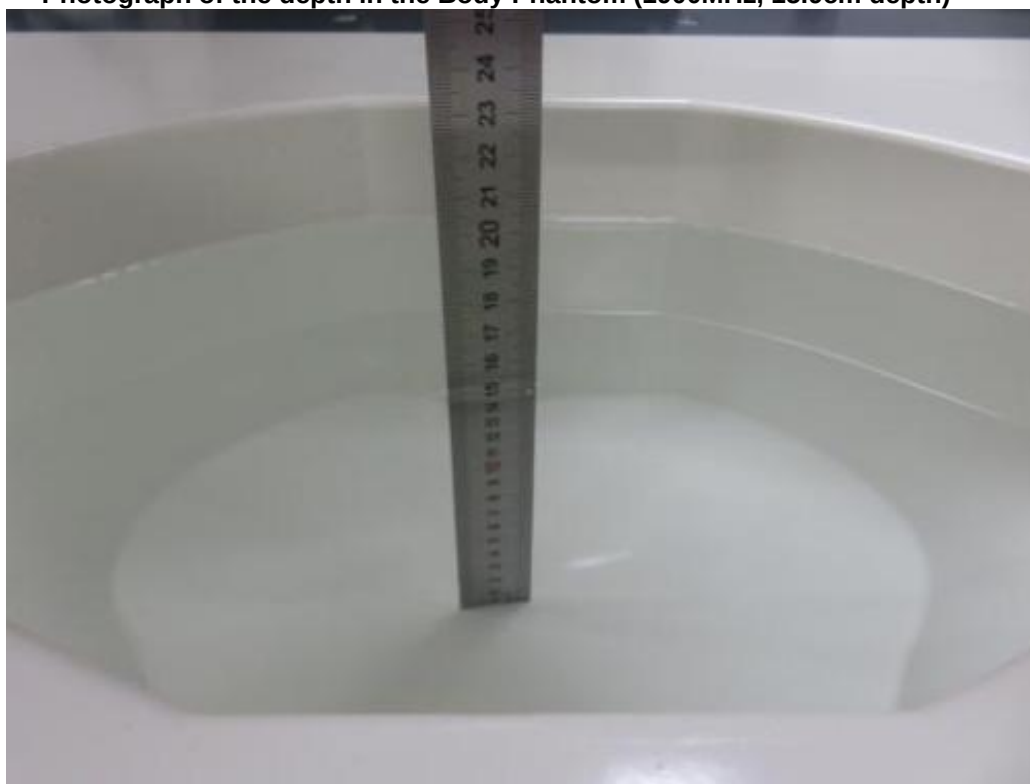
Photograph of the depth in the Body Phantom (1900MHz, 15.9cm depth)
