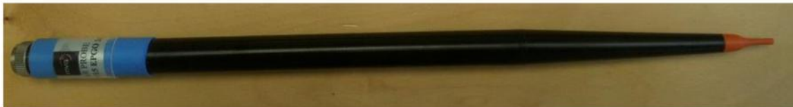
Figure 1 – MVG COMOSAR Dosimetric E field Dipole
