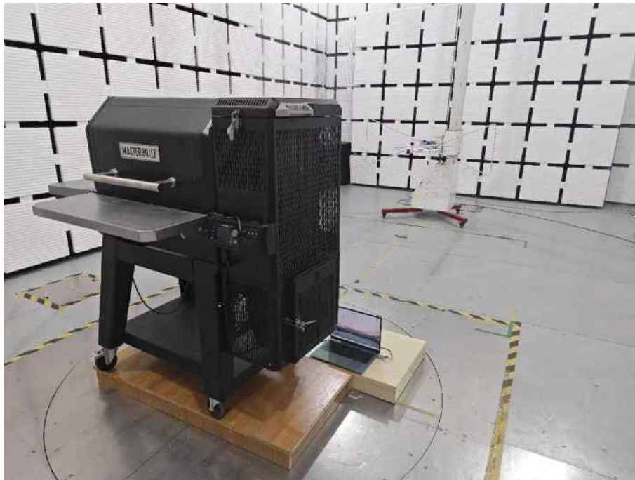
Set-up for Radiated Spurious Emission, Above 1GHz
