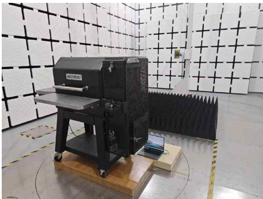
Set-up for Radiated Spurious Emission, Above 1GHz
