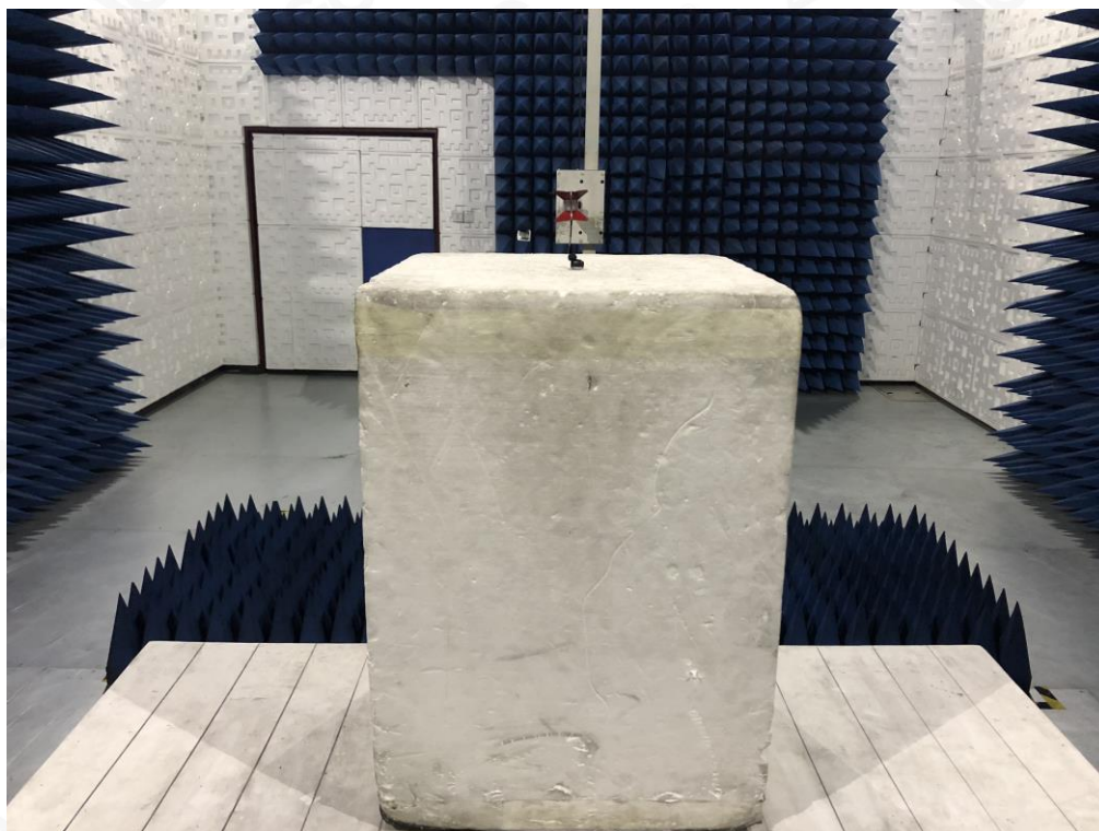
RADIATED EMISSION TEST SETUP ABOVE 1GHZ
