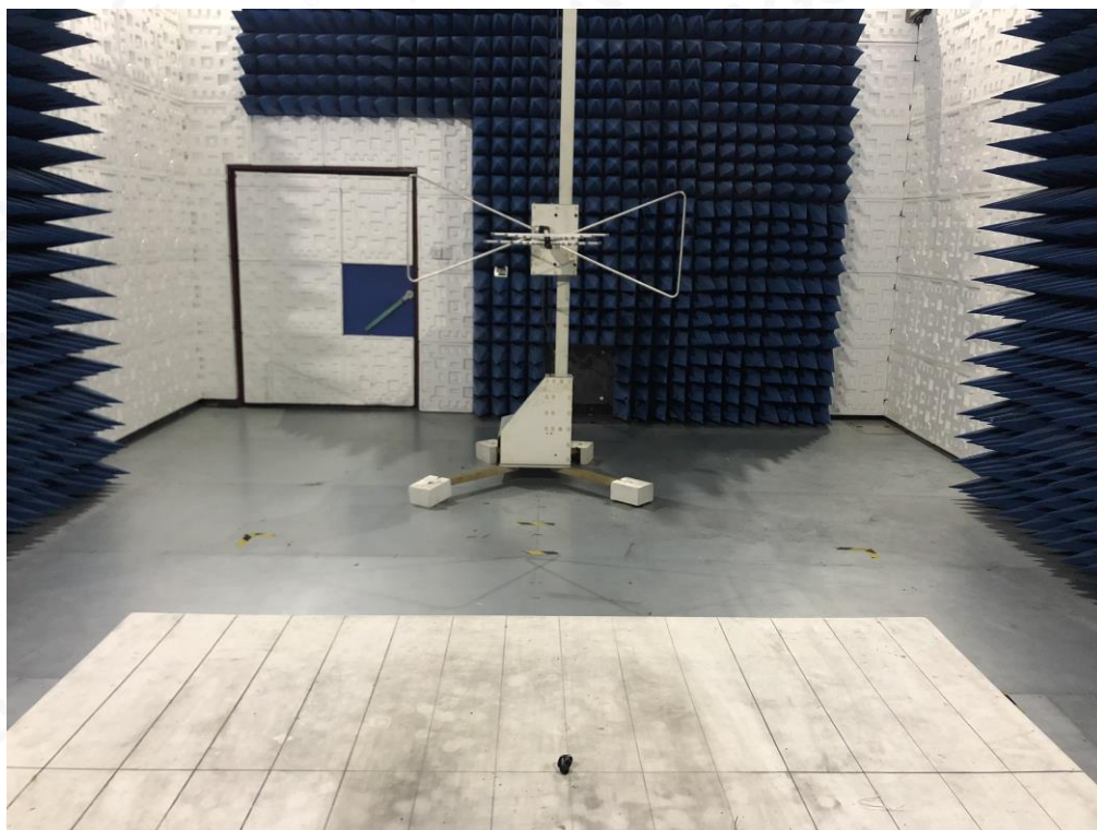
RADIATED EMISSION TEST SETUP ABOVE 1GHZ
