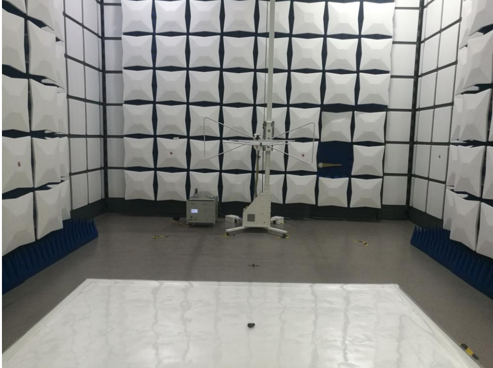
FCC RADIATED EMISSION TEST SETUP
