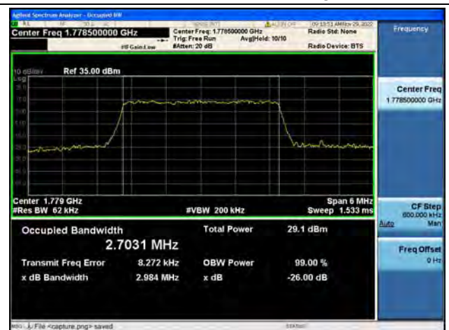
Band66 / 3MHz / 64QAM/ High CH
