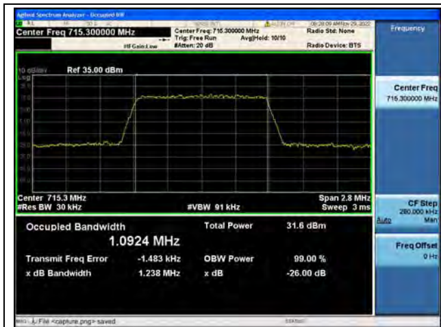
Band12 / 1.4MHz / QPSK/ High CH
