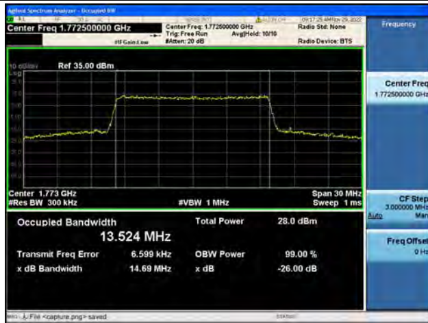
Band66 / 15MHz / 64QAM/ High CH
