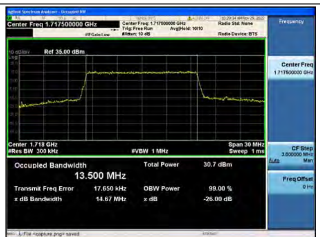
Band4 / 15MHz / 16QAM/ Low CH
