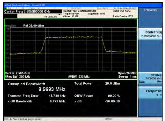
Band7 / 10MHz / 64QAM/ Low CH
