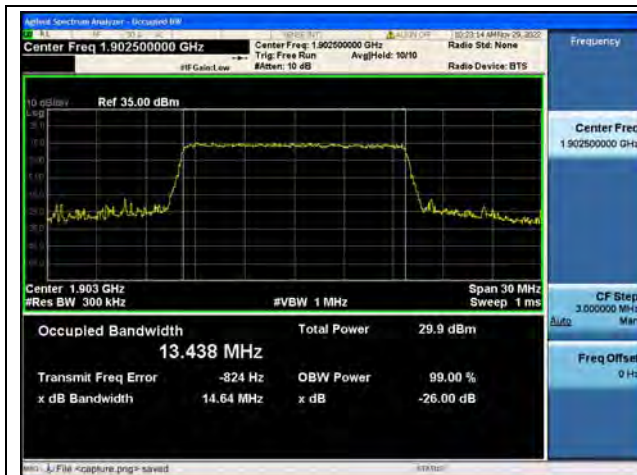
Band2 / 15MHz / QPSK/ High CH
