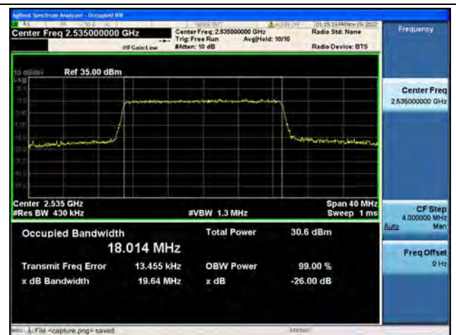
Band7 / 20MHz / 16QAM/ Mid CH
