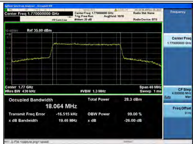
Band66 / 20MHz / 64QAM/ High CH
