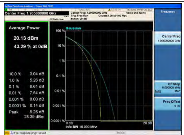
Band2 / 10MHz / High CH / 64QAM
