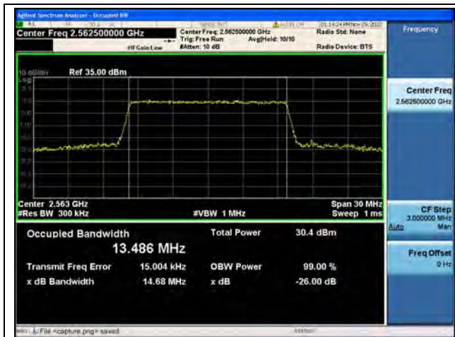
Band7 / 15MHz / QPSK/ High CH
