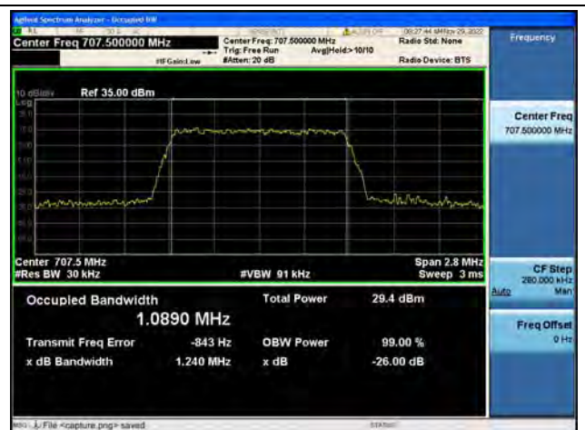
Band12 / 1.4MHz / 64QAM/ Mid CH
