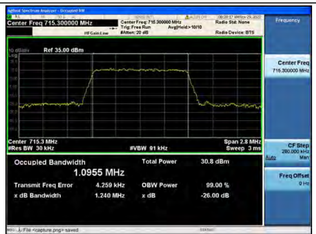
Band12 / 1.4MHz / 16QAM/ High CH
