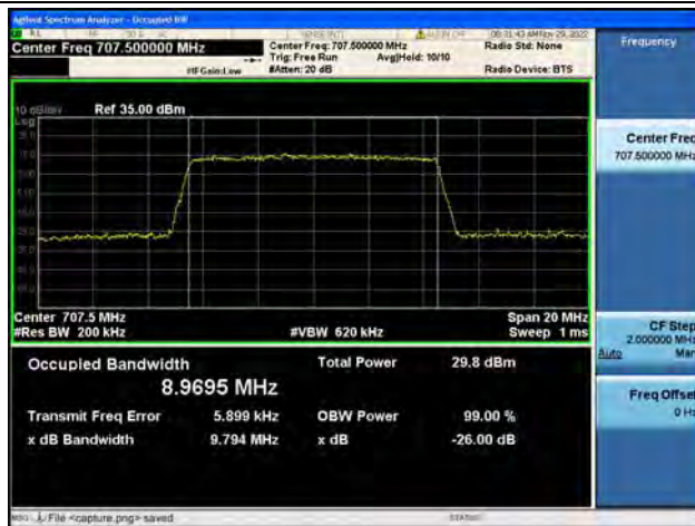
Band12 / 10MHz / 64QAM/ Mid CH
