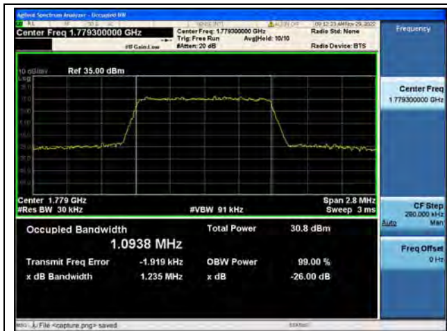
Band66 / 1.4MHz / QPSK/ High CH
