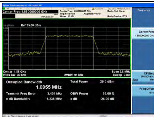
Band2 / 1.4MHz / 16QAM/ Mid CH
