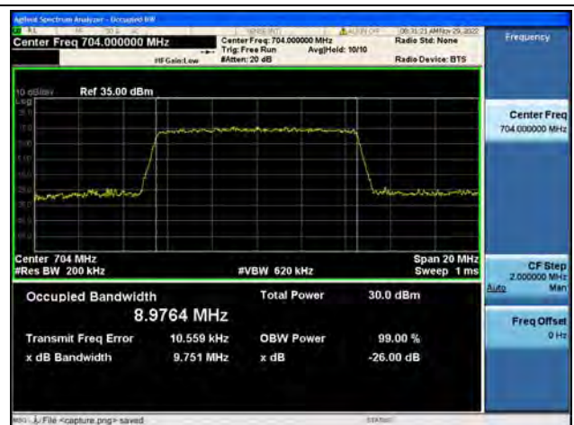
Band12 / 10MHz / 64QAM/ Low CH
