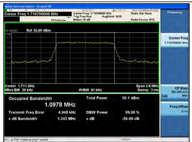
Band66 / 1.4MHz / 16QAM/ Low CH
