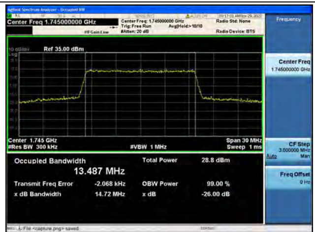
Band66 / 15MHz / 64QAM/ Mid CH
