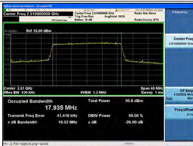
Band7 / 20MHz / 16QAM/ Low CH
