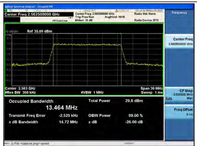
Band7 / 15MHz / 16QAM/ High CH
