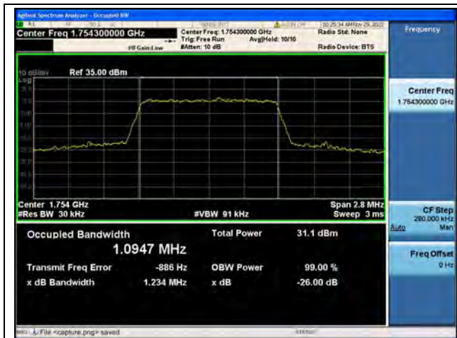
Band4 / 1.4MHz / QPSK/ High CH
