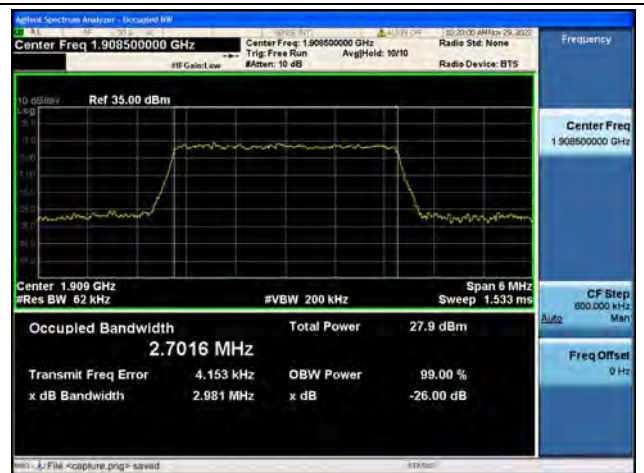
Band2 / 3MHz / 64QAM/ High CH
