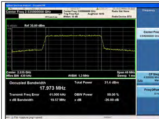
Band7 / 20MHz / QPSK/ Mid CH
