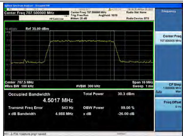
Band12 / 5MHz / 64QAM/ Mid CH
