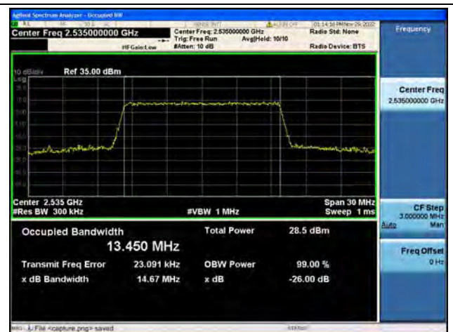
Band7 / 15MHz / 64QAM/ Mid CH
