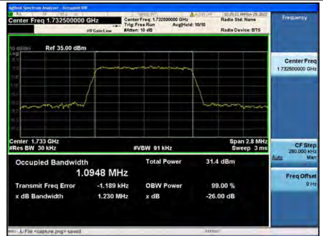
Band4 / 1.4MHz / QPSK/ Mid CH
