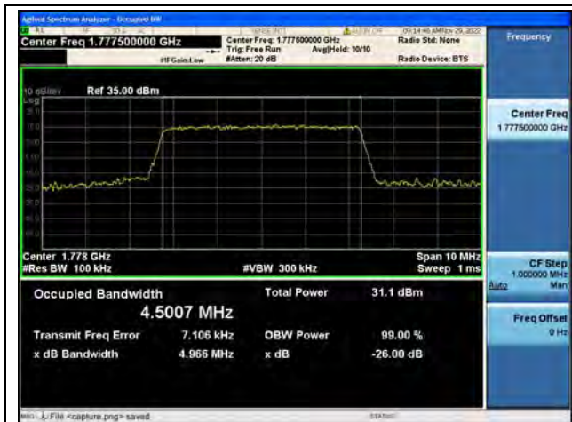
Band66 / 5MHz / QPSK/ High CH
