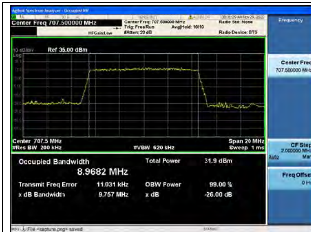
Band12 / 10MHz / QPSK/ Mid CH
