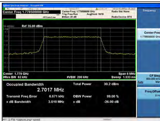
Band66 / 3MHz / 16QAM/ High CH
