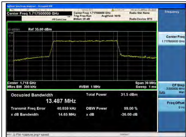
Band66 / 15MHz / QPSK/ Low CH
