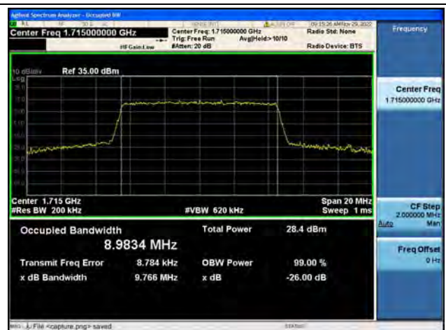
Band66 / 10MHz / 64QAM/ Low CH
