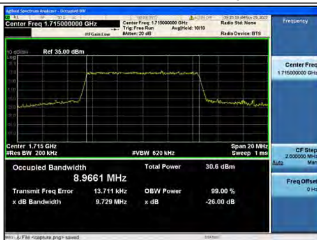
Band66 / 10MHz / 16QAM/ Low CH
