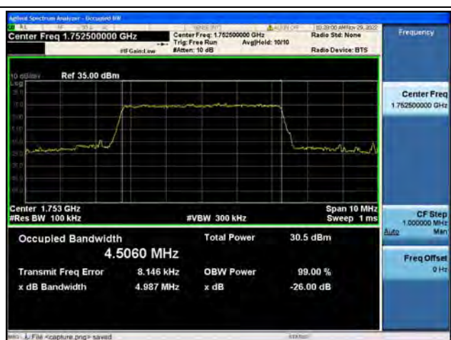
Band4 / 5MHz / 16QAM/ High CH
