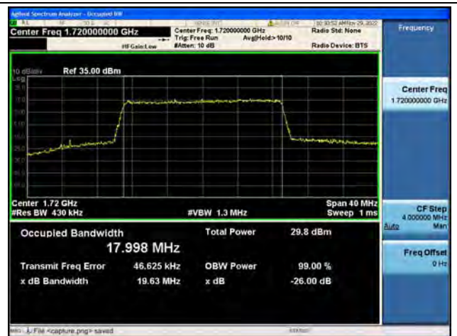
Band4 / 20MHz / 64QAM/ Low CH
