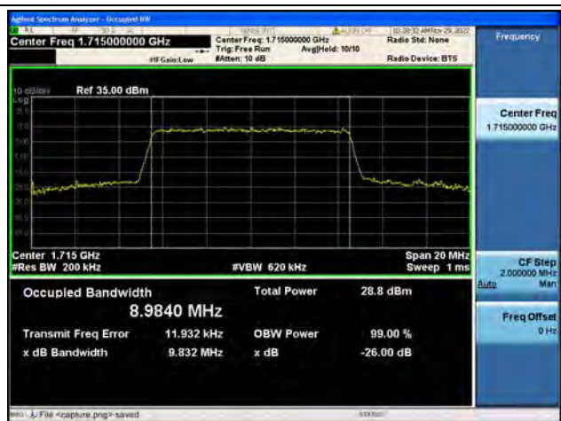
Band4 / 10MHz / 64QAM/ Low CH
