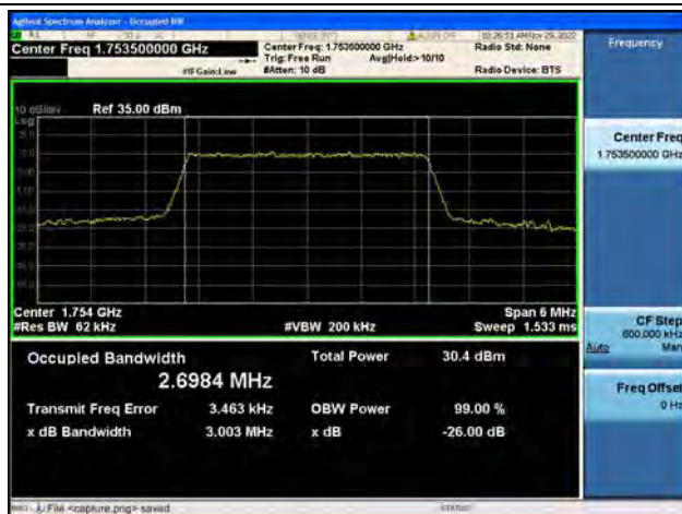
Band4 / 3MHz / 16QAM/ High CH
