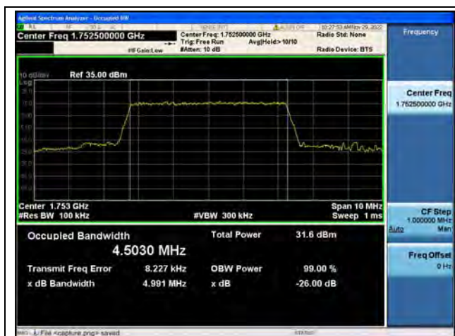
Band4 / 5MHz / QPSK/ High CH
