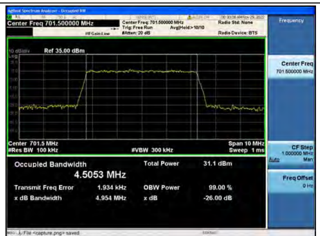
Band12 / 5MHz / 16QAM/ Low CH
