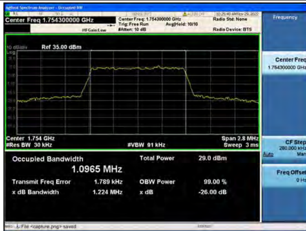
Band4 / 1.4MHz / 64QAM/ High CH
