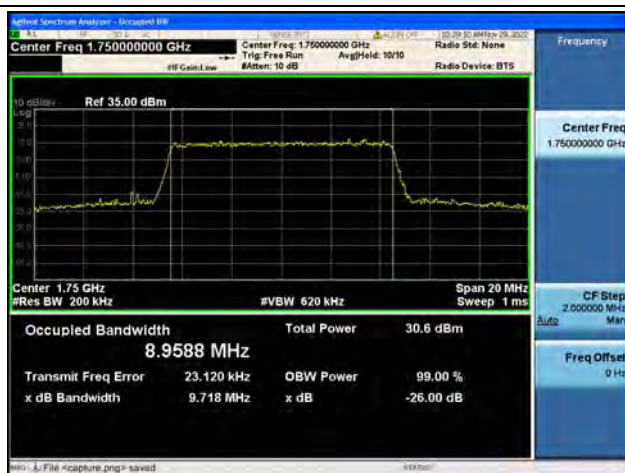
Band4 / 10MHz / 16QAM/ High CH
