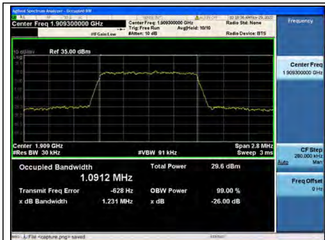
Band2 / 1.4MHz / QPSK/ High CH
