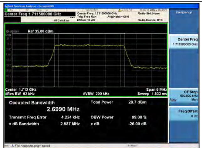
Band4 / 3MHz / 64QAM/ Low CH
