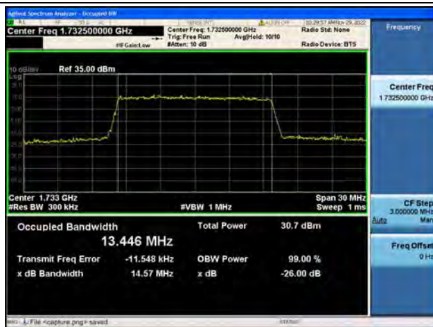
Band4 / 15MHz / 16QAM/ Mid CH
