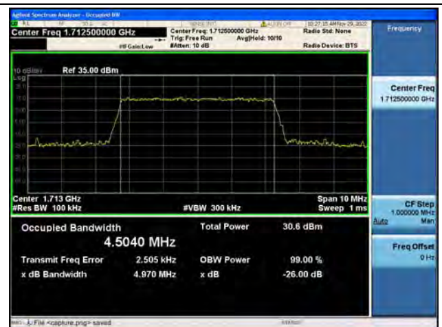
Band4 / 5MHz / 16QAM/ Low CH
