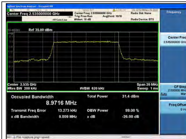
Band7 / 10MHz / QPSK/ Mid CH
