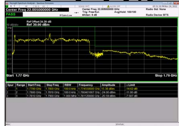
N66(10M)_DFT-s- OFDM QPSK Outer Full High CH
