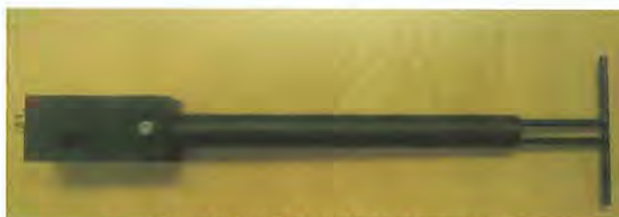
Figure 1 – MVG COMOSAR Validation Dipole
