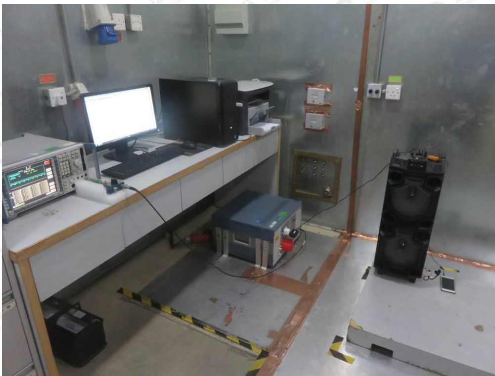
FCC RADIATED EMISSION TEST SETUP
